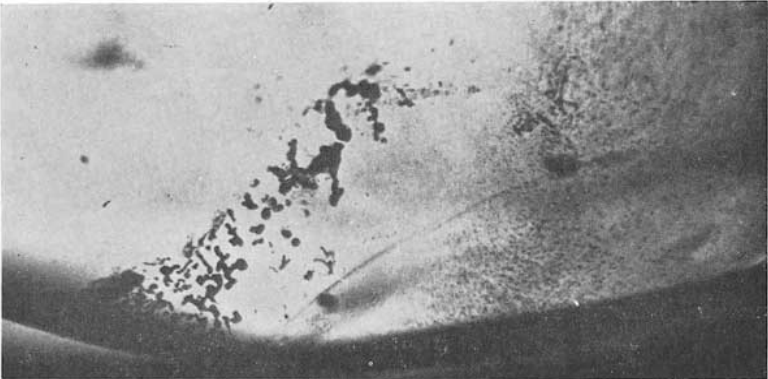
Bubble cloud and deceptive solid inclusions (probably alumina) in a synthetic ruby.
