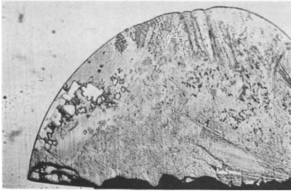
FIG. 34 Brown zircon from Madagascar. An epigenetic healing fissure, containing tiny droplets and some crystals (left). 120 ×
