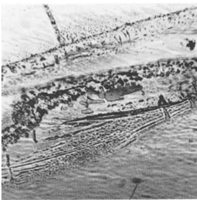
FIG. 21. Characteristic appearance and distribution of residual liquid drops in one of these tell-tale healing fissures in the hydrothermal overgrowth. Phase contrast 100 \times .
