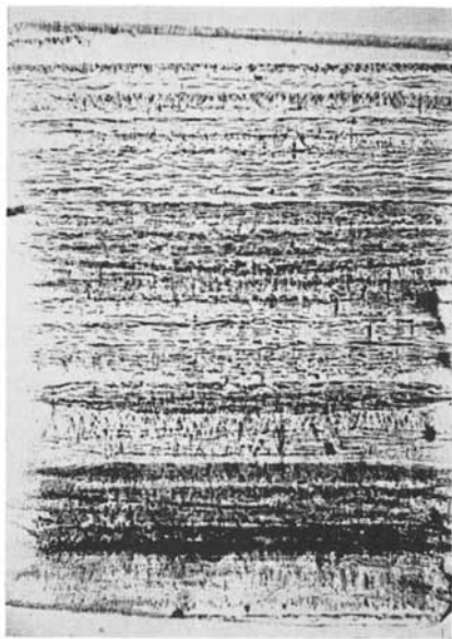
FIG. 2. Emerald with a marked striation parallel to the basal plane. Dark green layers alternate with brighter or colourless ones. 22 \times .
