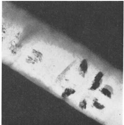
FIG. 10. Cracks (dark specks) in genuine beryl nucleus are mirrored in synthetic overgrowth if specimen is inclined and looked at through its body. Dark ground illumination. 40 ×.
