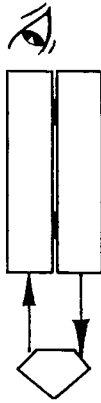
Spectroscope and electric battery lamp emitting focused light joined together to form the lighting spectroscope.
