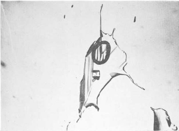
FIG. 5. Topaz of gem quality from Brazil, exhibiting a three-phase inclusion of irregular shape parallel to the basal plane. 120X
