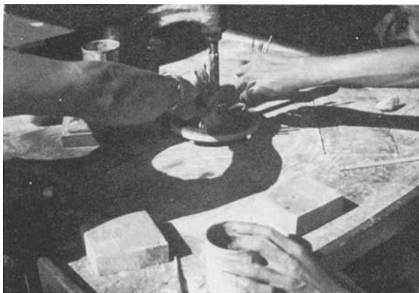
FIG. 17. Small rubies on thin sticks are worked into cabochons.
