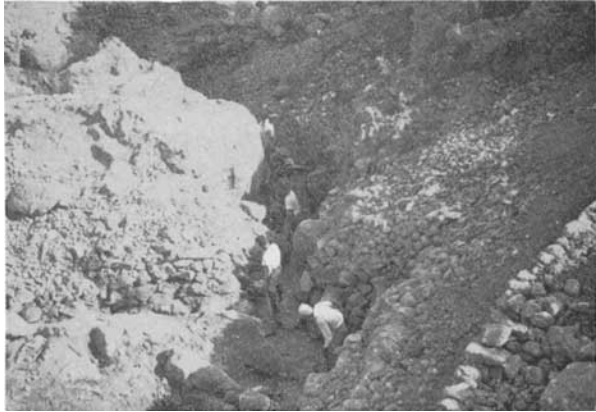
FIG. 5. The lower part of the valley is combed with many trenches in which the "byon" containing the rubies is carried and deposited in the lowest part of the mine.
