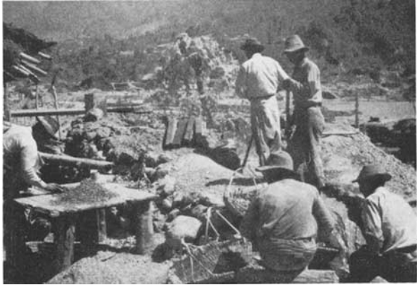
FIG. 11. A smaller working arrangement. The two men on top are roughly sorting the stones, the two lower men are washing the rubies and at the table sits the sorter.
