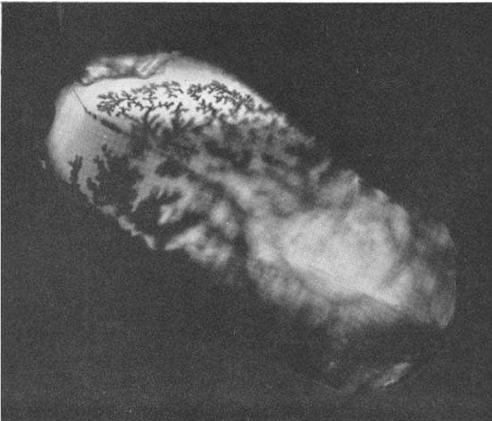
FIG. 4. Dendritic forms on crystal faces of one of the inclusions (190 ×).
