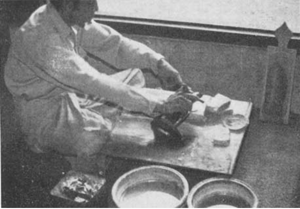
FIG. 19. The stone is rough-ground while being held in a primitive dop and rubbed on a carborundum-covered surface.
