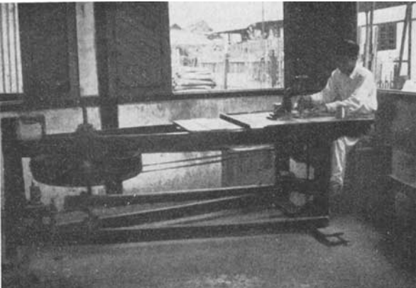
FIG. 21. Typical grinding wheel in Mogok. The wheel is rotated quickly by a treadle arrangement.
