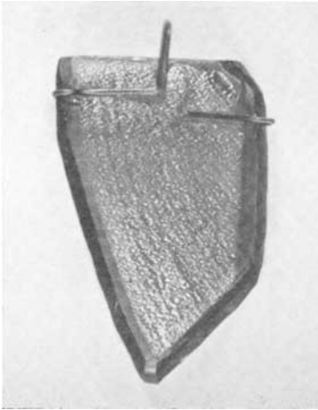
FIG. 3. Seed plate showing rough surface following one growth cycle. \times 3 (Photo Linde Co.).
