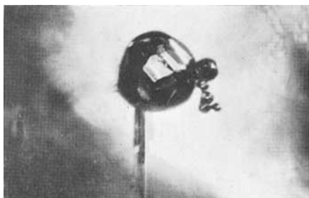
FIG. 1. Emerald from Burbar, Colombia. Crystals of pyrite from which a tube of growth started in the direction of the c -axis; reflected light. 120 \times
