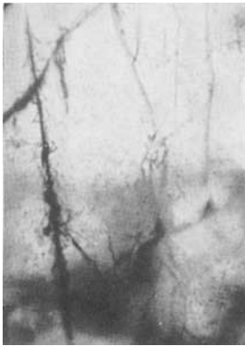
FIG. 3. Tube with jagged edges in Umba sapphire.
