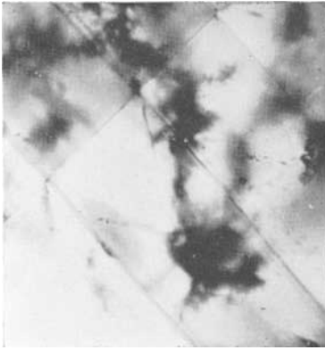
FIG. 1. Twinning planes in Umba sapphire.
