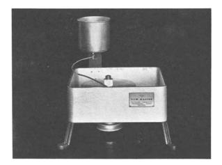
Three 6" diameter diamond-charged wheels are supplied with the machine, a coarse one for roughing out, a medium for shaping and a fine for semi-polishing. The life of these wheels is surprisingly long and only the coarse wheel is subjected to heavy wear. Even so, with moderate care, this wheel will last for the cutting of many hundreds of stones before it needs recharging and this can be done at a very nominal price.
