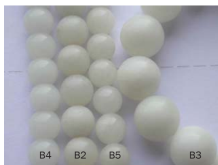
Figure 2: Sections of four strands of beads (of diameters between 8 and 12 mm) sample numbers B2, B3, B4 and B5. They are all pale grey and have a vitreous to waxy lustre that could easily be confused with white nephrite or some varieties of Shoushan stone. These strands of beads are identified as brucite (B2 and B3), glass (B4) and nephrite (B5). Photo by Li Jianjun.
