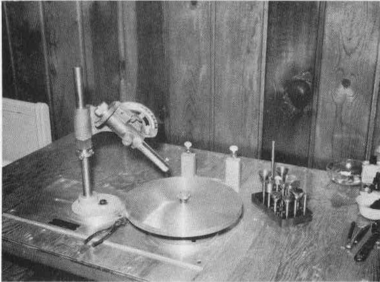
Figure 2 The specially made reproduction of the Allen Facet Unit used in cutting the spodumene. The splash pan is not installed. Behind the machine is the dop transfer jig; to the right are the dops. Photo courtesy Cedric Gleason
