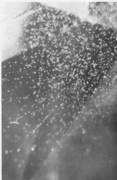
Pavilion of the synthetic sapphire showing the mass of gas bubbles and needlelike inclusion.
