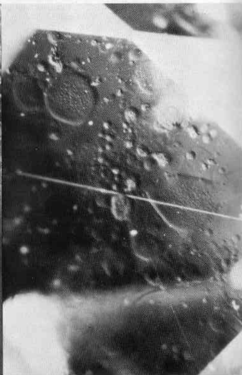
Crown facets of synthetic sapphire showing etched appearance and needlelike inclusion.
