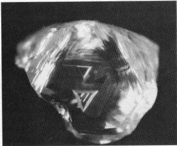
Trigon growth markings on the octahedral face of a small diamond
