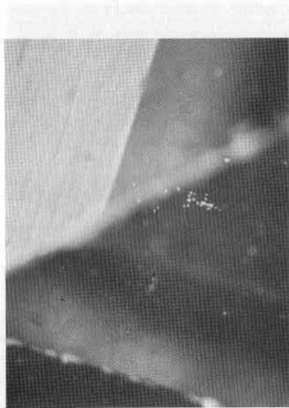
A group of gas bubbles in a synthetic ruby
