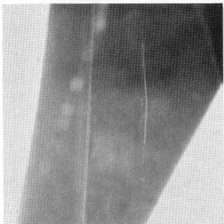
Figure 10 A needlelike inclusion (60x).
