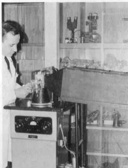
4. X-ray equipment for determining the origin of pearls and analysis of crystal powders.
