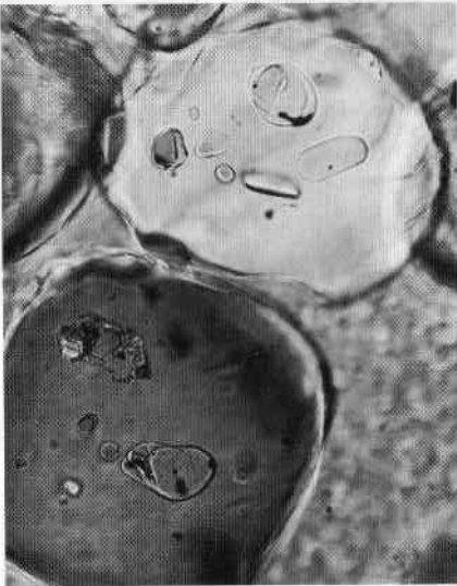
Figure 2 — Pseudo-isometric and rounded quartz inclusions showing in turn a variety of mono-phase inclusions. X-nicols. 0.2 mm. from face to face of the pseudo-iso shaped quartz crystal.
