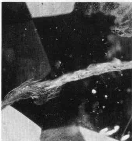
SYNTHETIC ALEXANDRITE. Coarse flux, hexagonal platelike inclusions, and wispy veil-like patterns are common.
