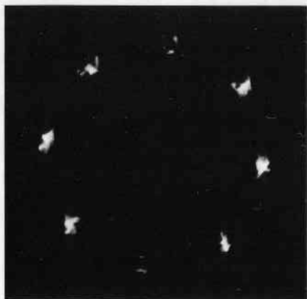
Fig. 1: Autoradiograph of the 1.16 carat radium treated diamond after 72 hours film exposure.
