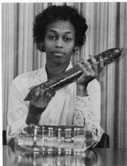
Figure 5. Czochralski-pulled synthetic ruby (4.2 kilograms, 9\frac{1}{4} pounds) and synthetic colorless sapphire (10 kilograms, 22 pounds). Courtesy of Union Carbide Corp.
