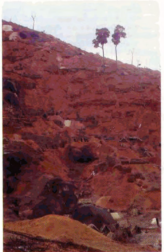
Figure 11. This hillside at the José de Sousa workings of the Três Barras deposit has been totally stripped by the hundreds of pits dug during the height of mining in this region (1968). Note the white kaolin dumps on the higher slopes, crescent-shaped series of tunnels into the colluvium, and the inselbergs, and garimpeiro shanties rising from the valley floor. Photo by Frederick H. Pough.
