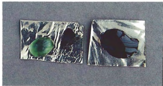
Figure 2. Left, the small, irregular pieces of green and black glass shown in figure 1 after heating to 800°C; right, the black glass heated to 1300°C.
