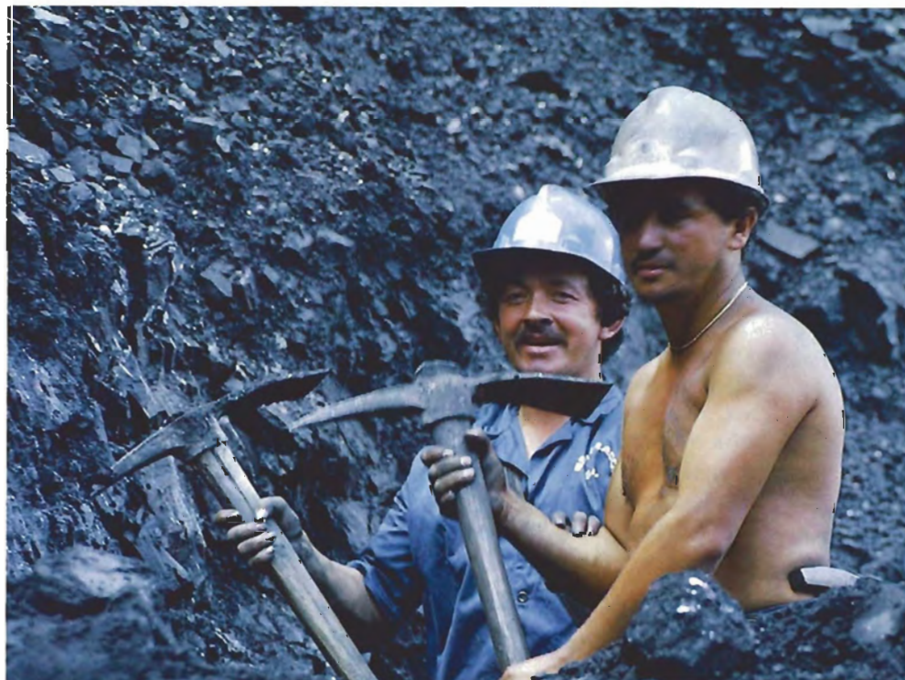
Figure 7. These Coscuez miners use picks to search for emeralds in the white calcite veins uncovered by the bulldozers.
