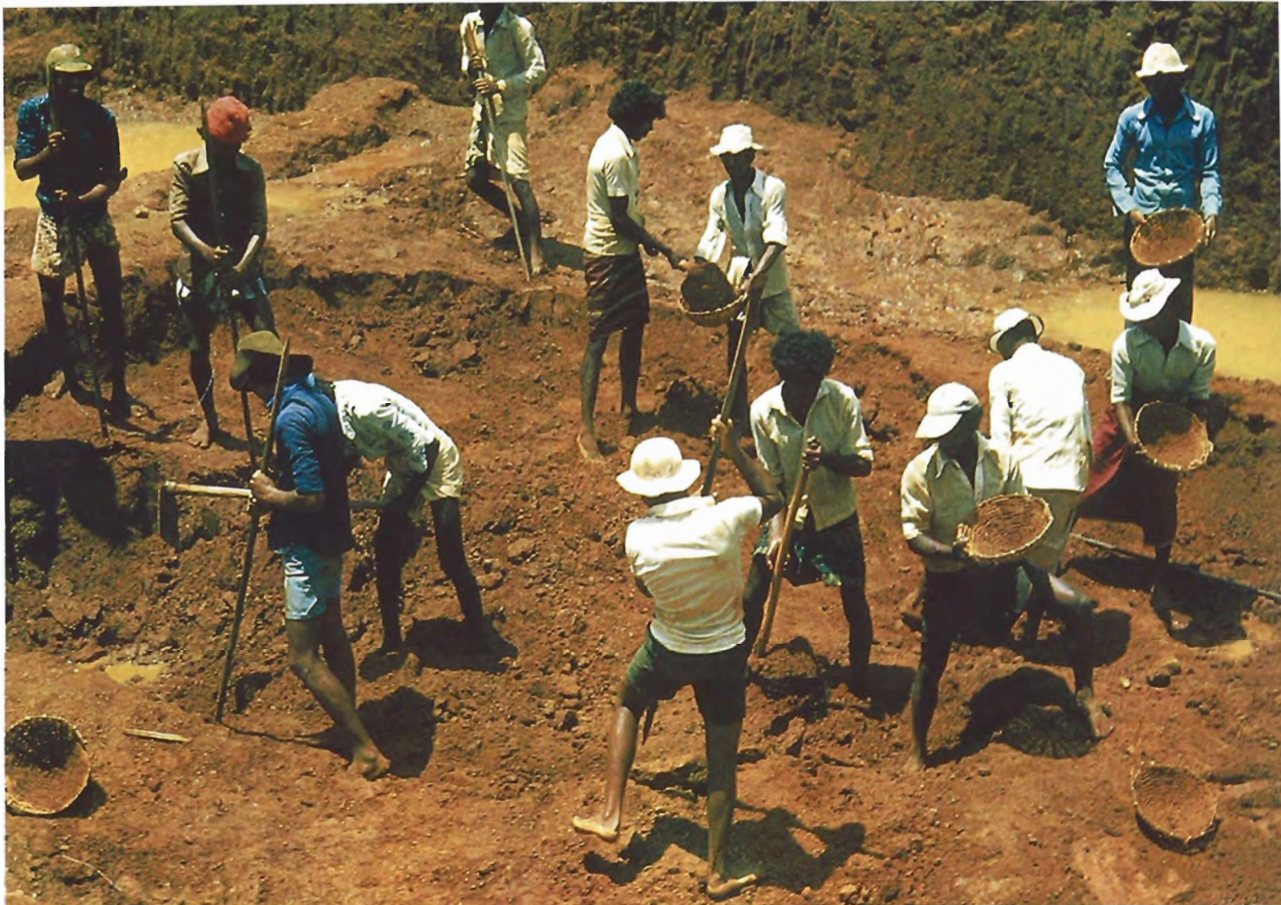
Figure 6. These surface-mining areas measure 20 to 30 m 2 . The earth is first excavated by bulldozers to a level just above the gem-bearing gravel. The workers then carefully loosen the gem gravel with picks and remove it in cane baskets. Photo by Marion Gunawardene.
