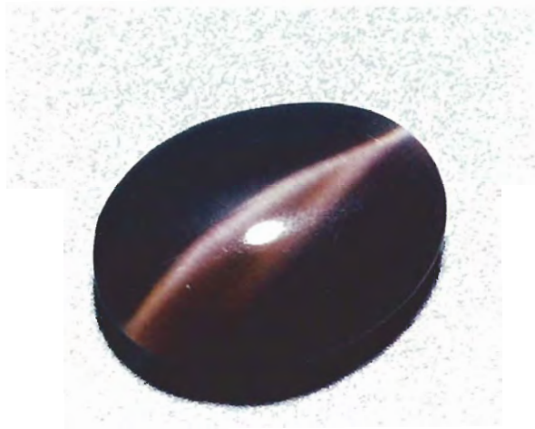
Figure 1. One of the sillimanite cat's-eyes from Sri Lanka that was studied by the authors. The relatively flat cabochon measures 13 mm and weighs 5.24 ct (although the stone originally weighed 10 ct, the base was cut off for the analyses). Note the bifurcated light band produced by irregularities in the orientation of the fibrous inclusions.
