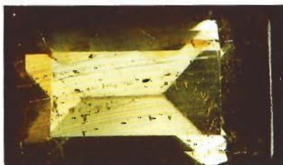
Figure 5. Curved color bands are seen here in natural andalusite. Magnified 20 \times .
