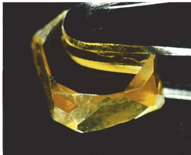
Figure 3. This is one of the larger pieces of Sumitomo synthetic diamond that is currently marketed for industrial applications. The piece has been cut from a single crystal such as the ones shown in figure 1. It weighs 0.37 ct and measures 3.7 \times 3.6 \times 1.7 mm. The large front and back surfaces have been sawn and polished. Various cube, octahedral, dodecahedral, or crystal faces that are modifications thereof, occur along the edge. Magnified 12 \times ; photomicrograph by John Koivula.
