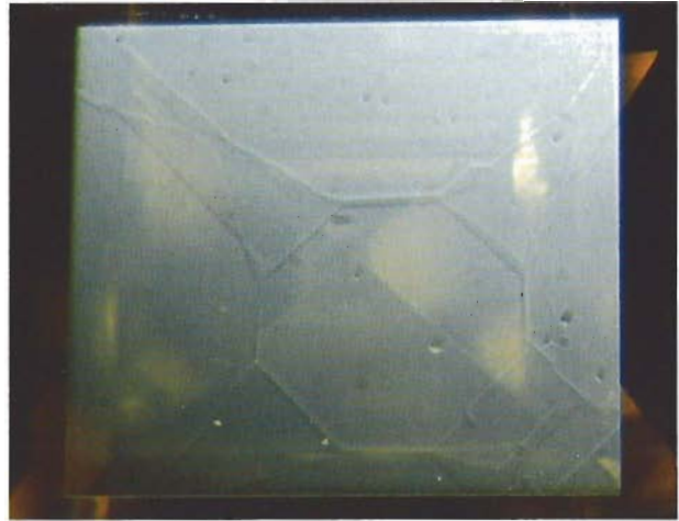
Figure 17. The surface grain lines shown here on one of the faceted stones reflect the external shape of the original Sumitomo synthetic diamond crystal. All of the faceted Sumitomo diamonds showed similar patterns on their tables. Oblique shadowed illumination, magnified 25 \times ; photomicrograph by John Koivula.
