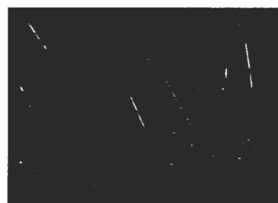
Figure 4. These spicules are the closest counterparts to the nailhead spicules typical of hydrothermal synthetic emerald that the lab has seen thus far in a synthetic amethyst. Magnified 20 \times .
