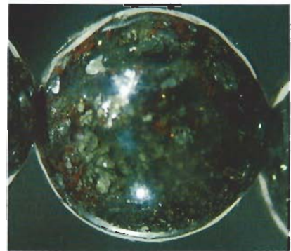
Figure 19. The quartz beads shown in figure 18 appear dark because of the heavy concentration of pyrite inclusions. Magnified 15x.
