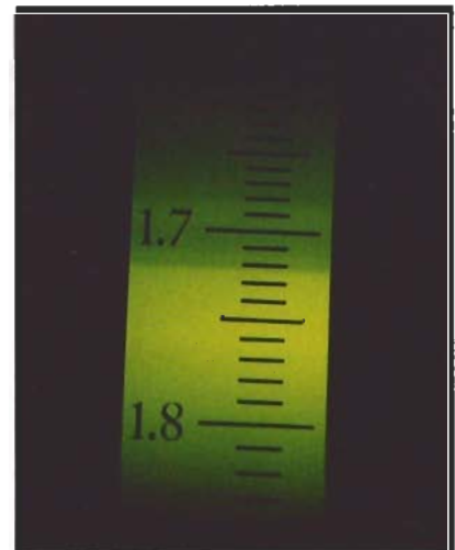
Figure 9. Multiple refractive index readings of synthetic spinel and the fused glass center.
