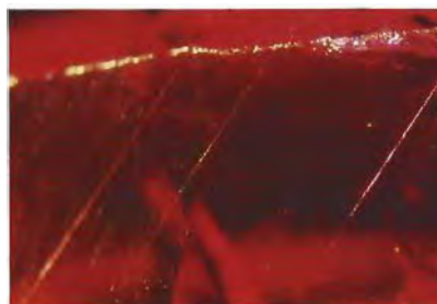
Figure 10. Straight twinning planes look like needles when viewed edge-on in this flame-fusion synthetic ruby. Magnified 45×.
