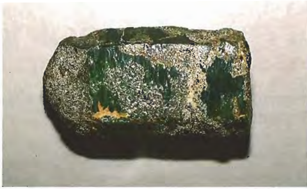
Figure 13. This 228.4-gram (1142-ct) quartz imitation of emerald proved to be a costly mistake for the person who purchased it in southern Africa. Photo courtesy of Dr. Henry A. Hänni.
