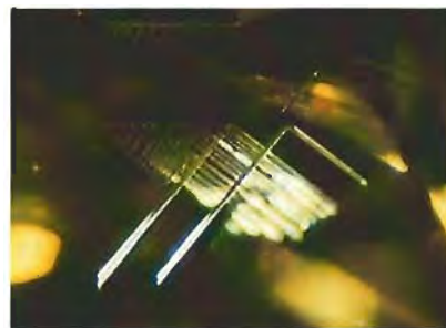
Figure 4. These sets of parallel "needles," which intersect at 90°, are unusual in diamond. Magnified 45 \times .
