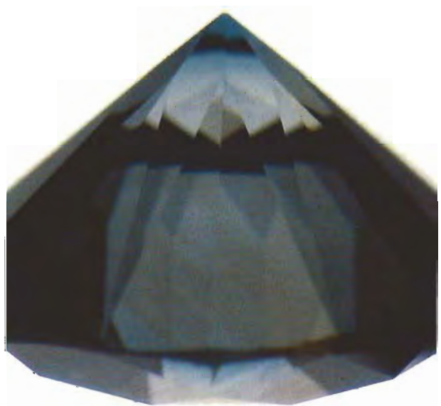
Figure 6. This treated blue diamond (sample 5), with a blue culet and light brown body color, is known to be electron irradiated. Photomicrograph by John I. Koivula.
