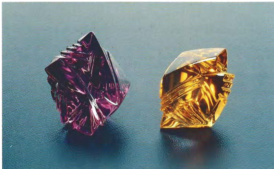
Figure 1. The 76.17-ct citrine on the right was originally the same color as its companion 89.26-ct amethyst. The color was changed by heat treatment. Photo by Bart Curren.
