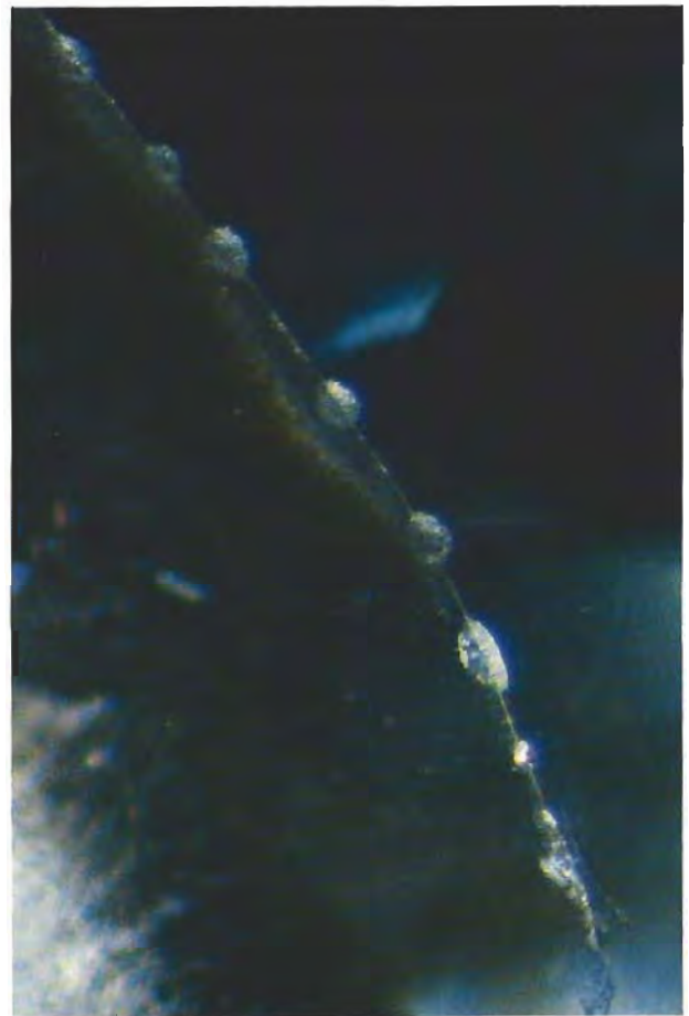
Figure 21. Beads of the filling agent can be seen as tiny droplets along the surface edge of the gap shown in figure 20. They sweated out during the retipping procedure. Magnified 50 \times .
