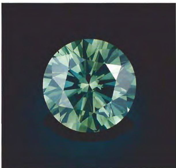
Figure 2. This treated diamond (sample 9) appears bluish green when viewed through the table. Photo by Robert Weldon.
