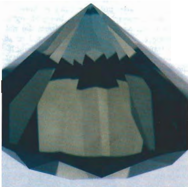
Figure 5. This treated bluish green diamond (sample 9, see also figure 2) displays a distinct blue zone at the culet. Photomicrograph by John I. Koivula.
