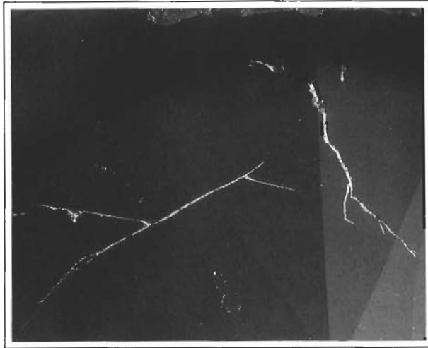
Figure 18. A scanning electron micrograph of filled breaks shows the very high contrast between the separation and the diamond. This indicates the presence of a foreign (noncarbon) material containing elements of high atomic number. Electron micrograph by John Armstrong; magnified 30 \times .
