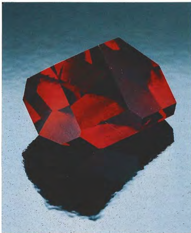
Figure 3. One of the attractive synthetics to reach the gem market in the 1980s is the Ramaura flux-grown synthetic ruby. This 23.86-ct crystal, the largest Ramaura rhombohedron grown to date, is courtesy of Ramaura Cultured Ruby, Judith Osmer; photo © Tino Hammid.
