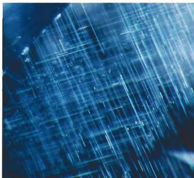
Figure 3. The distinctive rutile "silk" in a Sri Lankan sapphire before heat treatment (left) became stubby, partially absorbed, and dot-like (right) after the same stone was submitted to a heating procedure. Photomicrographs by John I. Koivula; magnified 30 \times .
