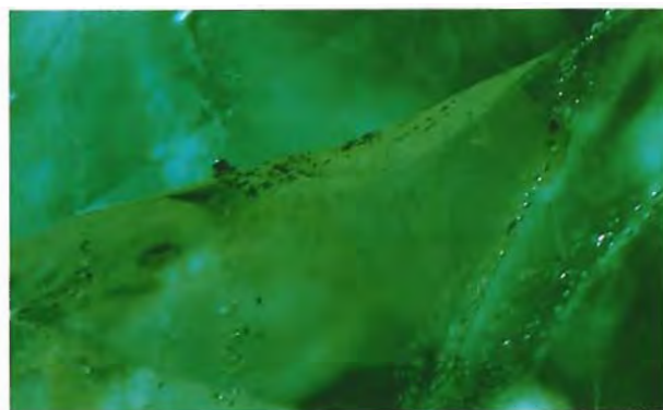
Figure 13. Colored oils, like that shown here in an emerald, may be detected as color concentrations in surface-reaching fractures. Photomicrograph by Robert E. Kane; magnified 25×.
