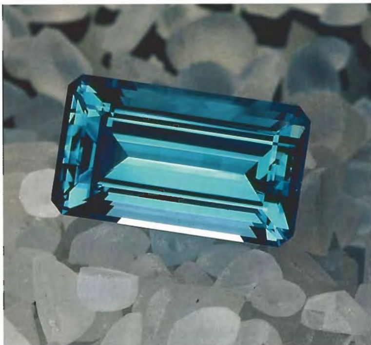
Figure 11. This 57.3-ct topaz derives its color from irradiation (in a linear electron accelerator) and subsequent heat treatment. It originally resembled one of the white topaz pre-forms on which it sits. Stones courtesy of P. Flusser, Overland Gems, Los Angeles, CA. Photo © Tino Hammid.
