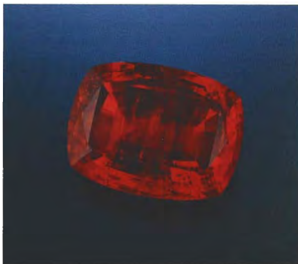
Figure 2. Large Knischka flux-grown synthetic crystals, like the one from which this 52.06-ct cushion cut was faceted, have been grown recently. Stone courtesy of P. O. Knischka; photo by Shane F. McClure.
