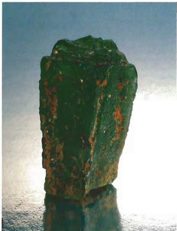
Figure 18. The five-sided symmetry quickly proves that this 34-mm-long fabricated glass specimen is not a natural beryl crystal. Photo by Robert Weldon.
