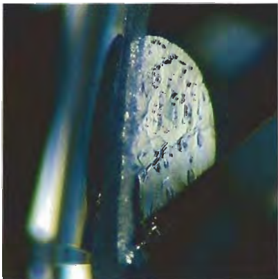
Figure 4. Darkfield illumination at 60× magnification shows what appears to be a cleavage in the girdle plane of a 1.53-ct diamond.
