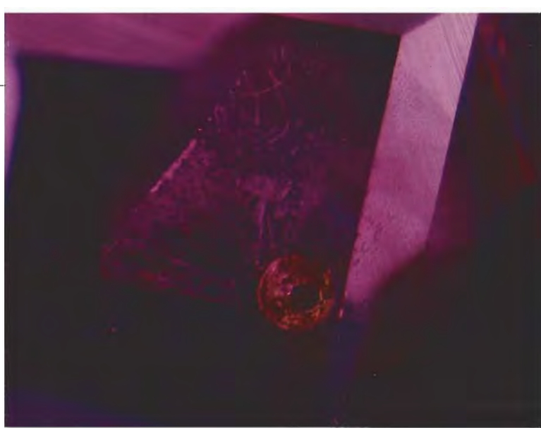
Figure 4. The lacy "fingerprint" surrounding a melted crystal inclusion in this Thai ruby is indicative of heat treatment. Photomicrograph by John I. Koivula; magnified 40 \times .
