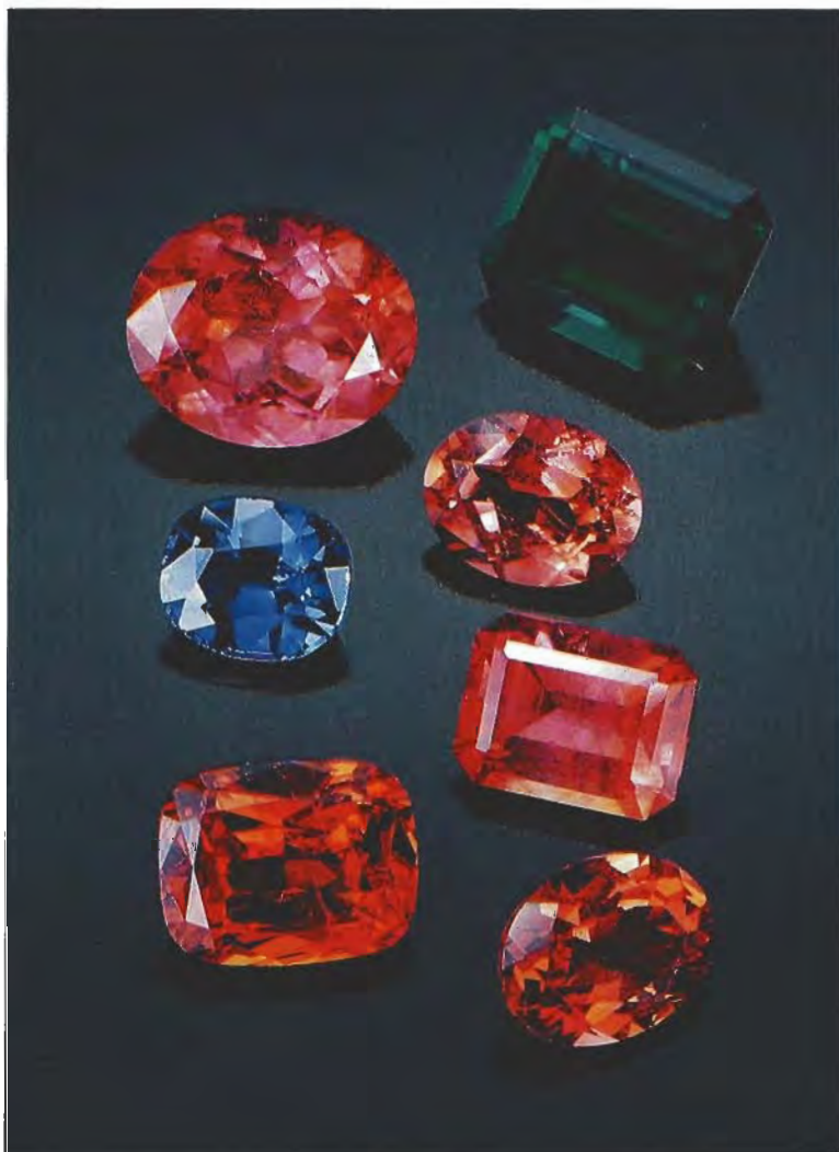
Figure 4. In the early 1980s, Chatham Created Gems, known for its production of flux-grown synthetic emeralds, introduced flux-grown blue, orange, and pinkish orange synthetic sapphires to the market. The Chatham synthetic emerald shown here weighs 4.15 ct; the synthetic sapphires range in weight from 1.91 to 6.20 ct. Photo © Tino Hammid.
