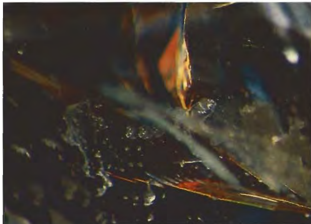
Figure 16. A "flash effect" is one of the most important visual features of filled separations in a diamond. In many fracture-filled diamonds examined to date, this effect is a characteristic yellowish orange in darkfield illumination (left); it changes to a distinctive blue when the stone is rotated slightly to a position where the background becomes bright (right). Photomicrographs by John I. Koivula; magnified 20 \times .
