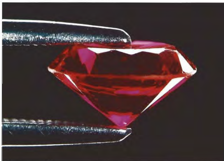
Figure 2. As part of the identification and evaluation of a gemstone, it is commonly held in the tweezers table-to-culet for examination through the crown and pavilion facets. Photomicrograph by John I. Koivula.
