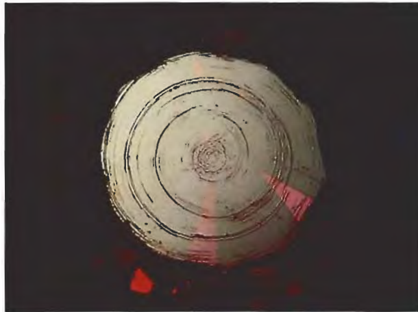
Figure 5. After only one 360° rotation in the jaws of the diamond-impregnated tweezers, considerable damage was done to the table facet of the synthetic ruby seen in figure 3. Photomicrograph by John I. Koivula; magnified 5 \times .
