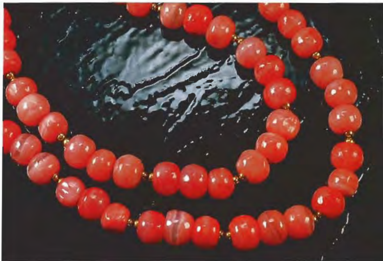
Figure 16. The 10-mm beads in this necklace resemble rhodochrosite but were determined to be dyed massive calcite. Photo by Robert Weldon.
