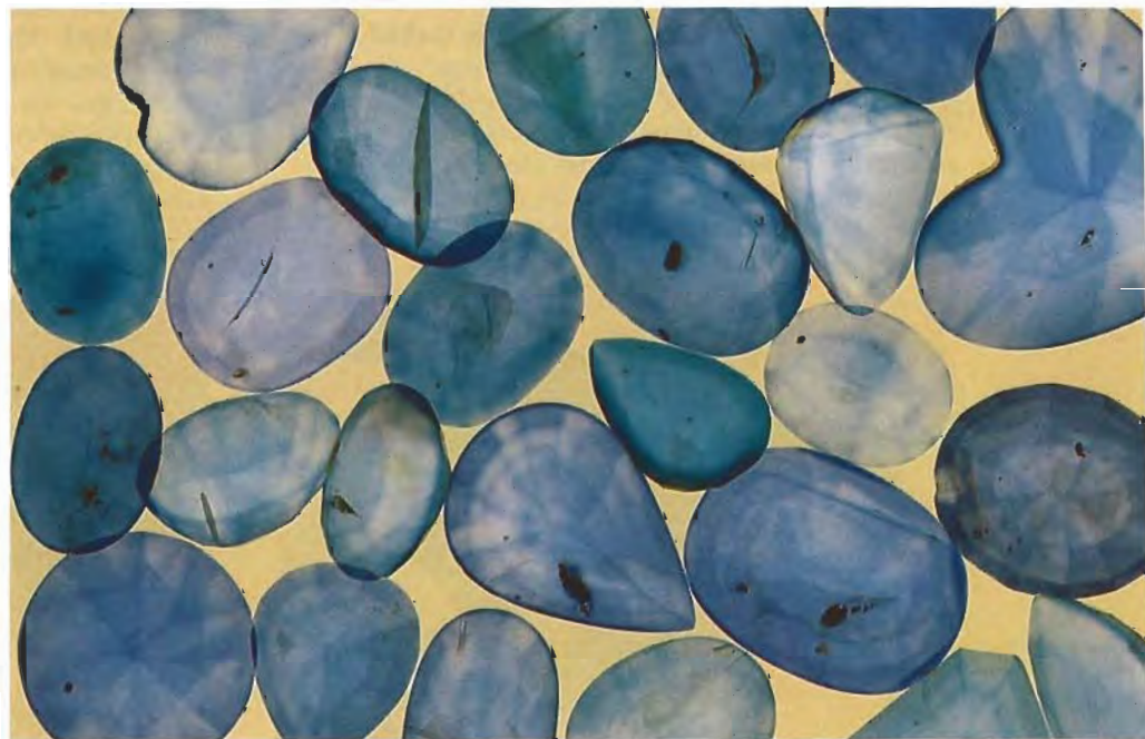
Figure 12. Immersed in methylene iodide over transmitted diffused illumination, this selection of diffusion-treated sapphires, from various "manufacturers," reveals the characteristic identifying features. These include: greater relief due to color concentrations at facet junctions, blotchiness of the diffused color layer, and areas without color. Photo by Shane F. McClure.
