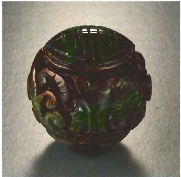
Figure 15. Sold as "jade" in Hong Kong, this carved sphere was determined to be a selectively dyed rock consisting of calcite and lesser amounts of serpentine. Photo by Robert Weldon.
