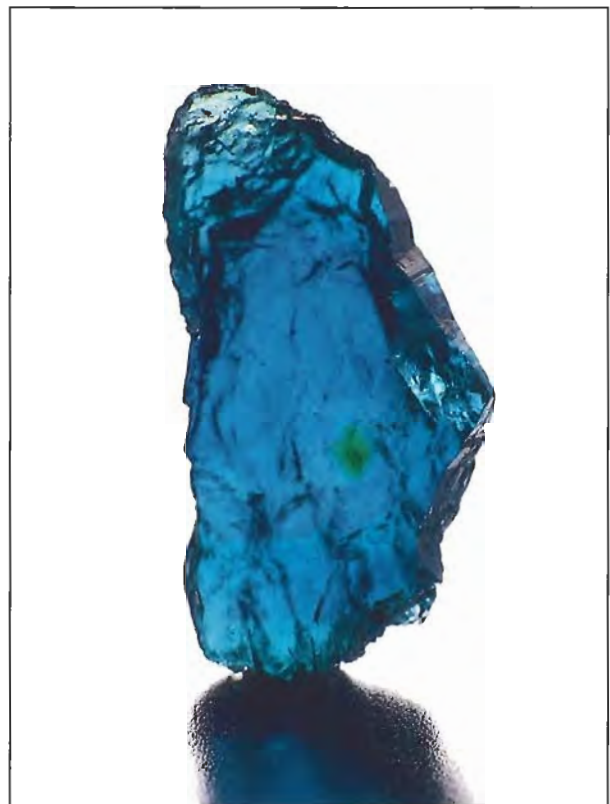
Figure 10. A needle of bright green tourmaline is readily seen as an inclusion in this slice of dark violetish blue tourmaline (R32) from Paraiba. The slice, 12.10 \times 6.60 \times 3.52 mm, is courtesy of Gerhard Becker; photo by Robert Weldon.
