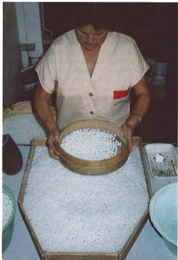
Figure 6. After the nuclei pass inspection, each "strand" is placed in an acid bath to remove the wire on which they were originally formed. Then, as shown here, the loose beads are sorted through sieves that place them into size categories with a tolerance of 0.2 mm. Photo by June Hanano.
