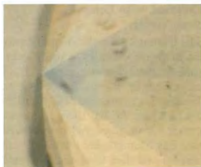
Figure 4. The zone of blue color around the culet of this diamond, seen here immersed in methylene iodide, shows that this bluish green stone had been subjected to electron irradiation. Magnified 6×.
