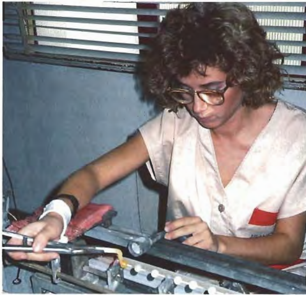
Figure 4. Although most nuclei are produced by Majorica's specialized machinery, those larger than 9 mm and those used to form pear-shaped beads are generally produced by hand. Today there are only a few women with the developed skill to make the near-perfect glass beads. Here, the technician controls the flame in one hand and manipulates the glass rod from which the nuclei are formed in the other. The end of the rod is worked under the flame until it begins to melt into a sphere onto a rotating wire. Photo by June Hanano.
