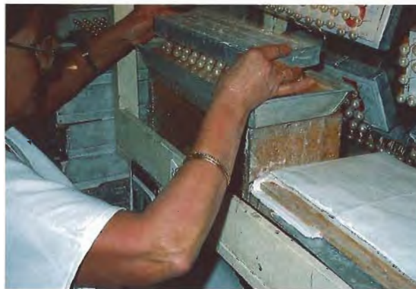
Figure 8. The glass bead nuclei are placed on posts in preparation for the coatings of “pearl essence.” They then undergo a series of dipping and drying steps, each followed by a cleaning and polishing. For the final coat, Majorica uses a special chemical that hardens the surface and protects the color from U.V. radiation. Although some beads are processed by hand, as shown here, most are done by automation. Photo by June Hanano.
