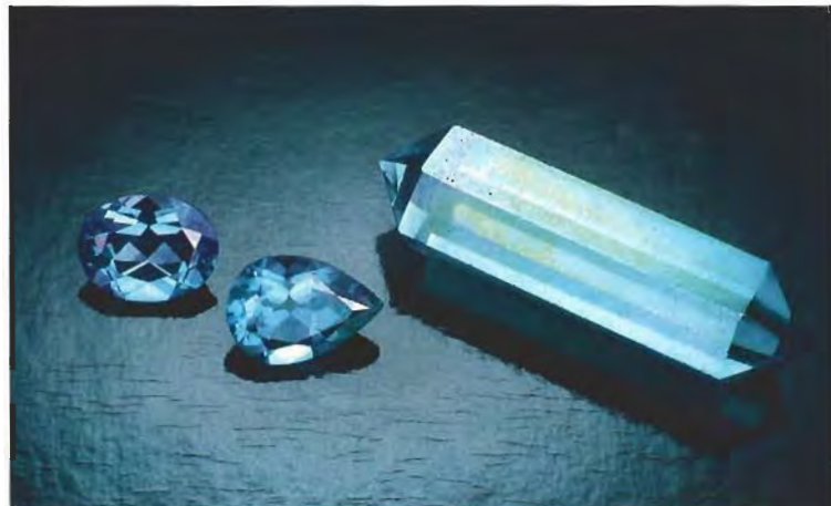
Figure 10. These two faceted topazes (the oval weighs 2.15 ct) and faceted hexagonal prism of quartz (18.18 ct) have both been treated by the Aqua Aura method. Photo by Robert Weldon.
