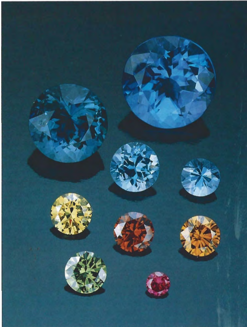
Figure 1. An important issue in gemology today is the presence of radioactivity in gem materials, especially that induced during color enhancement. Radioactivity is most commonly seen in irradiated blue topaz and colored diamonds. The four topazes at the top (0.52–7.87 ct) and the five diamonds at the bottom (0.10 [reddish purple stone] to 0.52 [yellow] ct) in this suite are known to be irradiated. The four topazes are still very slightly radioactive. Photo © GIA and Tino Hammid.
