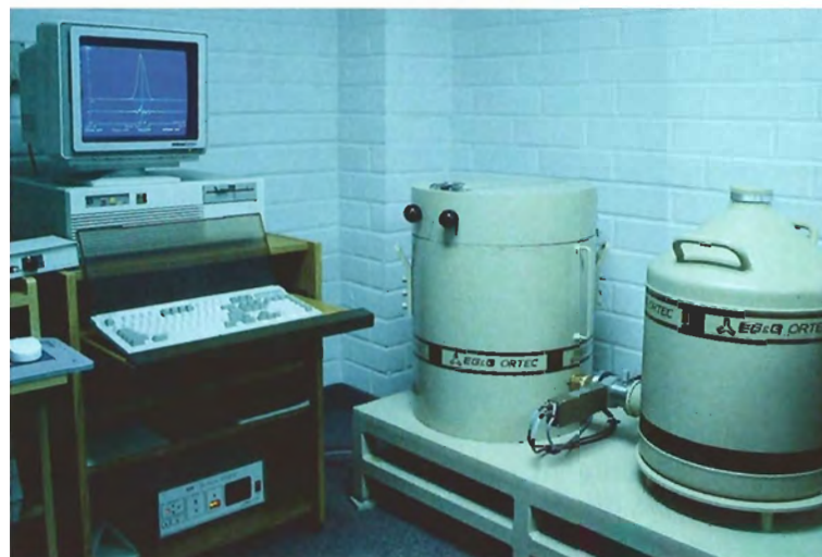
Figure 4. The high-purity (intrinsic) germanium (HPGe) gamma-ray spectroscopy system at the GIA radiation testing facility includes, from left to right: a computer, associated electronics, a 2,000-lb. graded lead shield (which houses the germanium crystal detector), and a liquid-nitrogen storage tank. Gamma rays from the sample stone are absorbed by the germanium crystal, which then produces minute electrical pulses that are amplified and sent to a computer for analysis. This system was manufactured by EG&G Ortec. Photo by Maha Smith.
