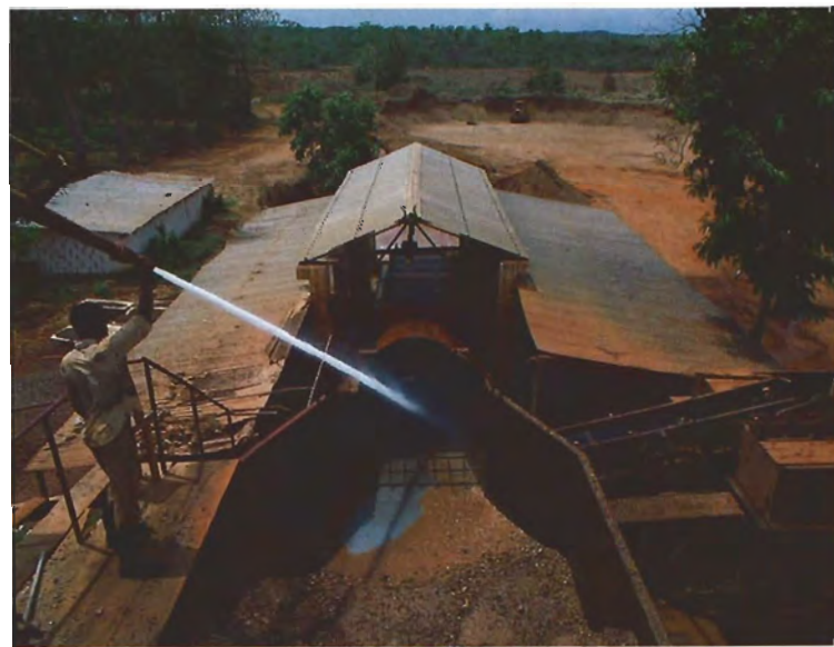
Figure 5. This mechanized washing plant serves a ruby mine located about one hour south of Mahenge that is operated by Simba International Investments Ltd. Using the diesel motor of a truck, the miner washes the gem-bearing gravels before they are sent to the jigs for final separation of the rubies. Photo © Fred Ward.
