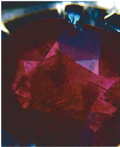
Figure 17. Sharply curved striae and dark inclusions, seen here at 19×, prove that the synthetic rubies shown in figure 16 are of early manufacture.
