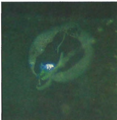
Figure 7. High magnification (126x) revealed that what was believed to be "jardin" in an emerald is actually a combination of bubbles and flux in a green YAG.
