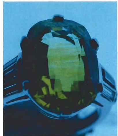
Figure 19. Curved striae are easily visible without magnification in this 15.50 x 10.75 x 6.15 mm flame-fusion synthetic yellow sapphire.
