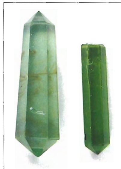
Figure 9. These two glass imitations (note the stretched gas bubbles in the larger one) were sold as "healing crystals." The larger piece measures 34.16 x 10.10 x 9.27 mm.
