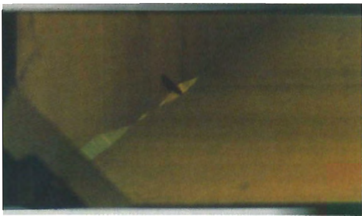
Figure 9. In Sample 1, a narrow, near-colorless-to-blue {110} zone points toward a corner of the sample. Brown graining runs parallel to two sides of the crystal that are cube faces. The elongated flux inclusion appears to be oriented parallel to one of the crystal faces. Photomicrograph by John I. Koivula; magnified 75 \times .
