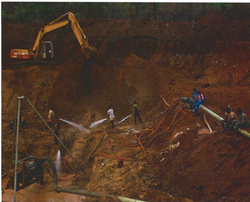
Figure 11. In the valley of the Umba River, mechanized mining is now used to recover corundum and associated gems from the rich gem gravels. Photo © Fred Ward.
