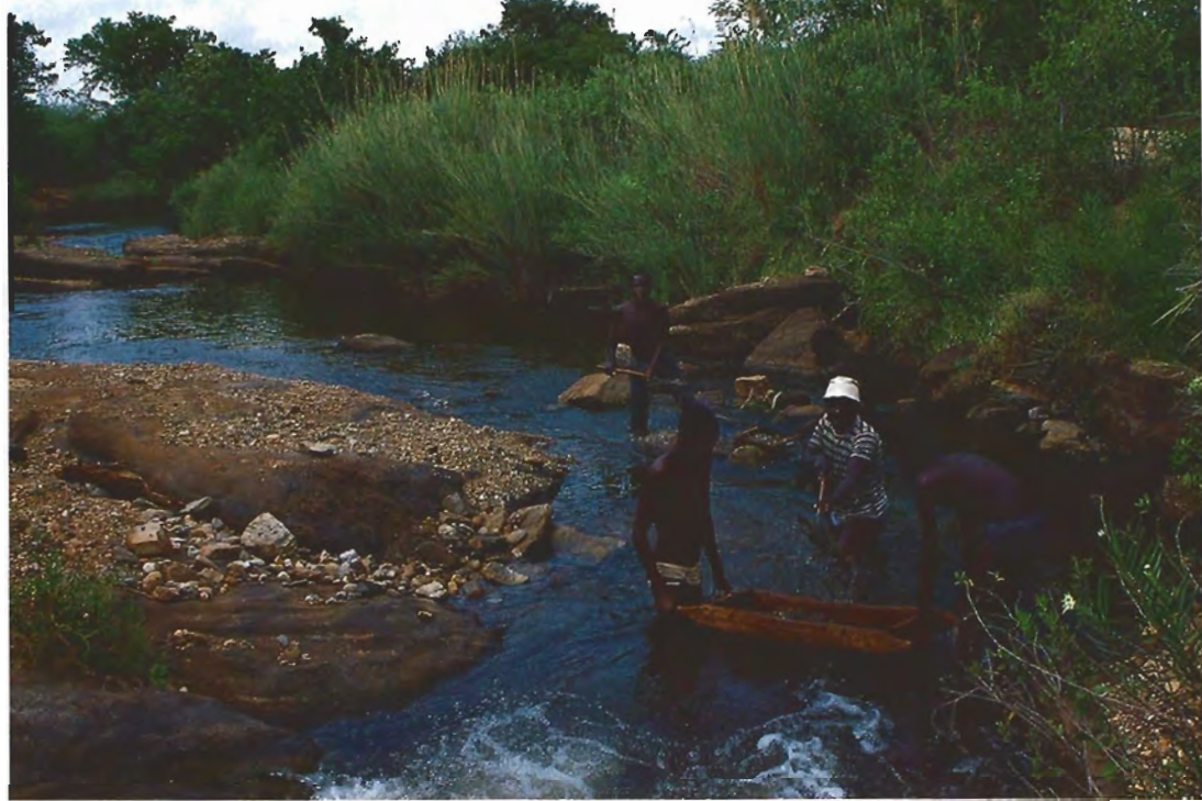
Figure 4. Much of the mining in Tanzania is alluvial, often secondary deposits along streambeds. Here, miners use rudimentary shovels and screens to locate corundum and other gems in the gravels of the Umba River. Photo © Fred Ward.
