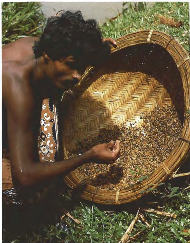
Figure 2. A miner examines river gravel for various types of rough. Most "prospecting" in Sri Lanka to date has been by independent miners, who search broad areas using only shovels and washing baskets. Photo by Robert C. Kammerling.
