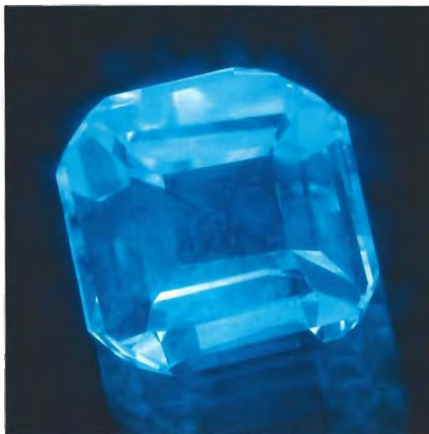
Figure 7. The uneven cathodoluminescence of the smaller GE ^{12}\text{C} synthetic diamond results from the conditions of crystal growth, which produced an arrangement of octahedral and cube internal growth sectors that are revealed by their differing luminescence behavior. Photo by Maha DeMaggio.
