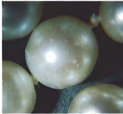
Figure 14. The central areas of these pearls (5.6–10.4 mm in diameter) have been eroded by contact with the acidic skin of the wearer. Magnified 10 \times .
