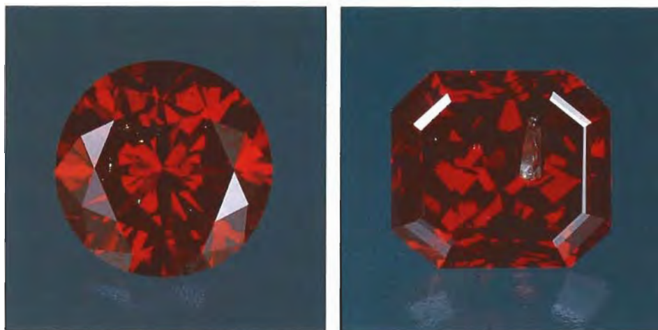
Figure 1. Standard gemological testing at the GIA Gem Trade Laboratory in New York revealed that this 0.55-ct brownish orangy-red round brilliant cut (left) and this 0.43-ct brownish red "radiant" cut (right) are synthetic diamonds that have been treated to produce the red color. Photos by Shane F. McClure.
