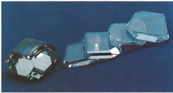
Figure 3. One of the new GE ^{12}\text{C} synthetic diamond crystals is shown here cut into slices for use in various high-technology applications. Photo courtesy of General Electric.
