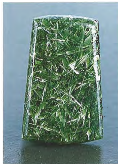
Figure 8. This unusual 12.25-ct tablet, which is reminiscent of a mass of actinolite crystals, proved to be devitrified glass.
