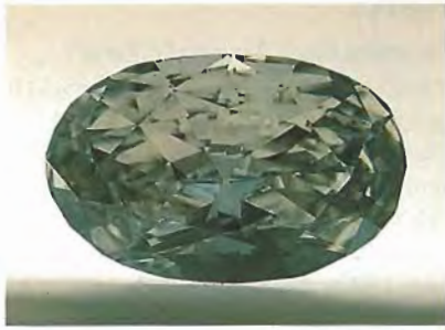
Figure 6. A small blue color zone, present on only one side of the culet of this 0.75-ct oval diamond, not only strongly influences the stone's faceup color, but also proves that it has been treated.
