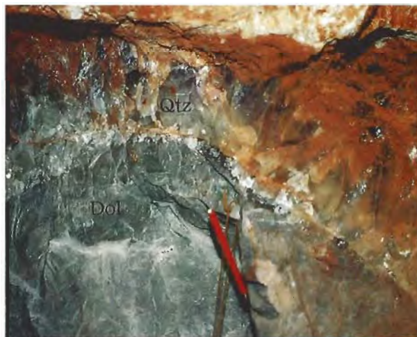
Figure 5. Quartz (Qtz) precipitates on the walls of vugs formed by dolomite (Dol) brecciation. Because these dolomite blocks are massive, they are routinely blasted to allow access to new pockets. At the contact with the dolomite, quartz is microcrystalline; it becomes coarse crystalline and milky away from the contact, and it eventually forms euhedral crystals with tips that are purple and orange-yellow. The quartz-bearing cavities are often filled with clay minerals. Photo by P. Vasconcelos.
