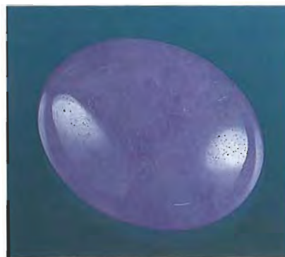
Figure 9. Infrared spectroscopy confirmed that this 15.86-ct lavender jadeite cabochon had been polymer impregnated.
