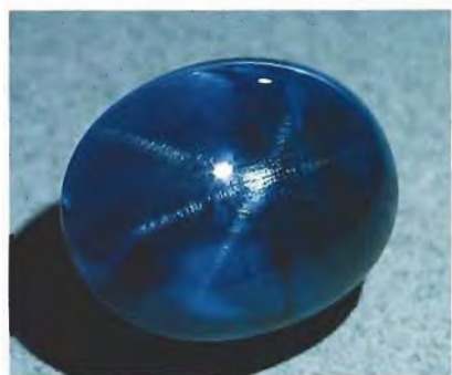
Figure 18. Face up, this 11.66-ct blue star sapphire displays asterism, as well as some brilliancy that is not usually seen when a standard cabochon cut is used for such material.
