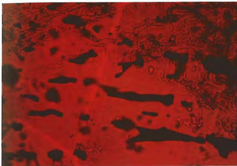
Figure 7. Note the coarseness of the residual flux in this overgrowth on a Lechleitner synthetic ruby. Photomicrograph by K. Schmetzer; immersion, magnified 100 \times .
