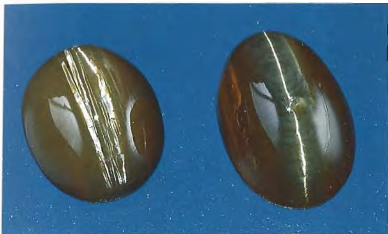
Figure 9. Before it was soaked in water for several minutes, the 1.74-ct cat's-eye opal on the right looked almost identical to the 1.40-ct untreated stone on the left. Stones courtesy of Jean-Claude Nydegger; photo by Shane F. McClure.
