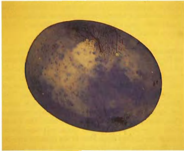
Figure 4. When the stone shown in figure 3 was immersed in methylene iodide, color concentrations along facet junctions were noticeably absent but the facets revealed a dimpled appearance. Photo by Tony Laughter.
