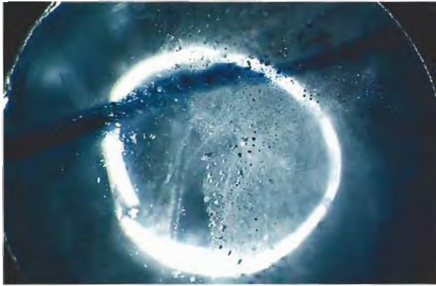
Figure 14. "Bleeding" of diffused color can clearly be seen in this 0.15-ct sapphire cabochon. The stone had been "salted" into a parcel of natural sapphires from Kanchanaburi and was subsequently repolished. Courtesy of Mark H. Smith, Bangkok; photomicrograph by John I. Koivula, magnified 10 \times .
