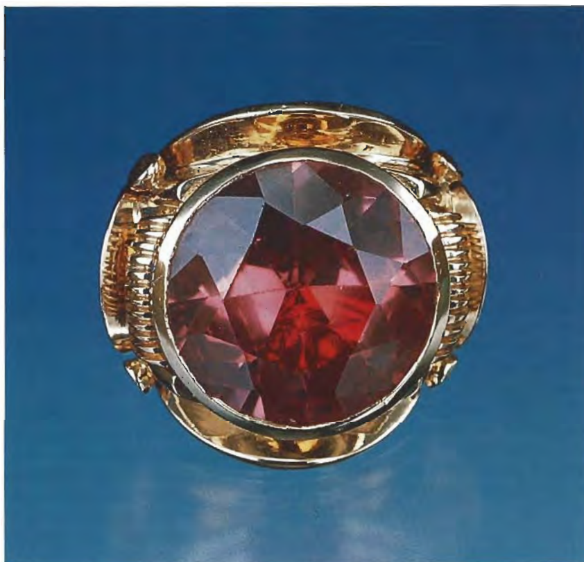
Figure 20. Face up, this 15.80-mm color-change synthetic sapphire appears redder than is typical for this material because of a coating on the pavilion facets.
