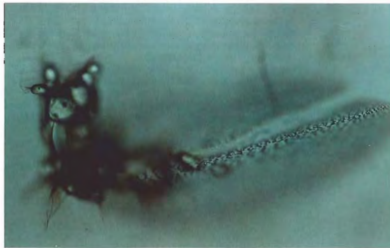
Figure 9. This brown-stained inclusion looks like zircon. Note the tension halo associated with a healed fracture. Photomicrograph by J. C. Mendes; magnified 200 \times .
