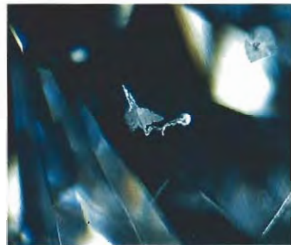
Figure 3. The somewhat irregular laser drill hole in this 4.69-ct diamond travels from the table to a crystal and feather inclusion. Note the cone-shaped opening. Magnified 27×.
