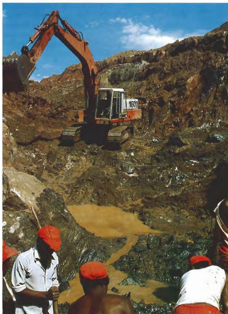
Figure 4. At Morafeno, this mining company uses a backhoe to reach the emerald-bearing schists. Photo by E. Julius Petsch, of Julius Petsch Jr., Idar-Oberstein.
