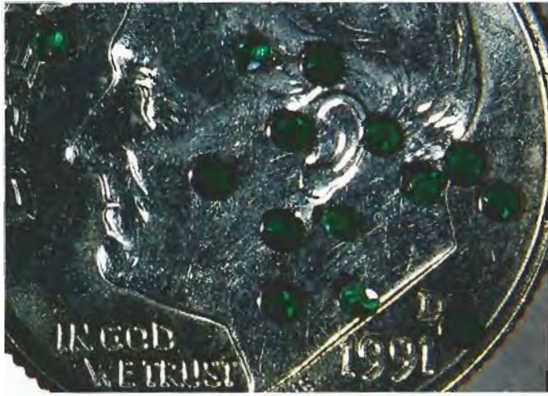
Figure 15. These 1.15-mm synthetic spinel triplets are representative of some of the tiny synthetics and simulants now being fashioned with robotic cutting. Photo by John I. Koivula.
