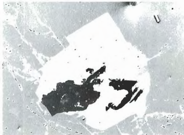
Figure 11. The intergrowth of quartz (black) and carbonate (white) inclusions in Mananjary emeralds is readily apparent in this scanning electron micrograph. Magnified 200×.
