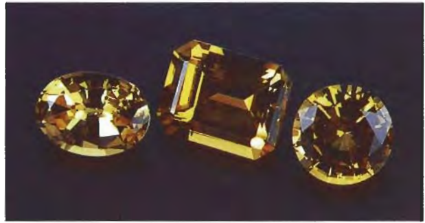
Figure 18. Nickel is the primary coloring agent in these three synthetic sapphires (1.66, 2.91, and 1.66 ct) produced by the Czochralski-pulling method. Courtesy of Manning International; photo by Maha DeMaggio.
