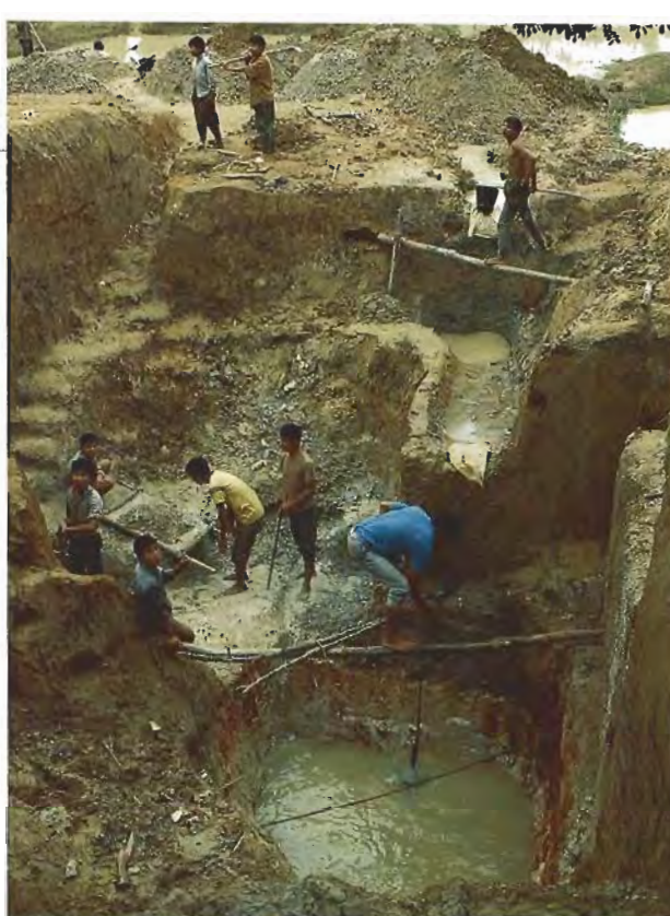
Figure 7. Most of the mining operation of Company No. 2, located at Quy Chau's "Millionaire Hill," was being done by hand. Some of the miners reached the gem-bearing gravels by digging large pits like that shown here. Photo by Robert C. Kammerling.
