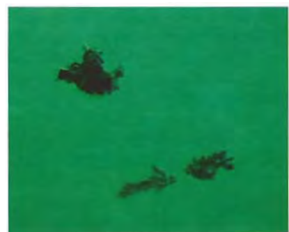
Figure 10. Some of the inclusions in the stone shown in figure 9, seen here with darkfield illumination, appear to be brown when viewed in reflected light. They may be pyrrhotite. Magnified 30×.
