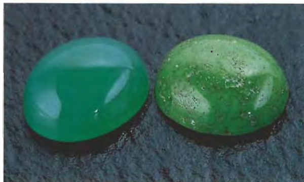
Figure 6. The cabochon on the left (2.65 ct, 8 × 10 mm) is chrysoprase chalcedony from Queensland, Australia; the other (3.15 ct, 8.22 × 10.13 mm) is gaspeite, a nickel ferrous carbonate mined in Western Australia. Photo by Maha DeMaggio.
