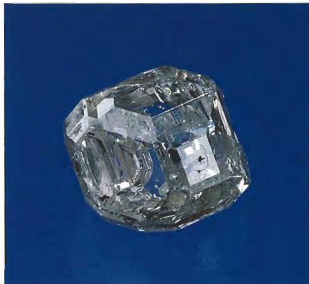
Figure 1. This 0.42-ct near-colorless synthetic diamond crystal was produced in Russia by means of a belt apparatus. Courtesy of Chatham Created Gems; photo by Shane F. McClure.
