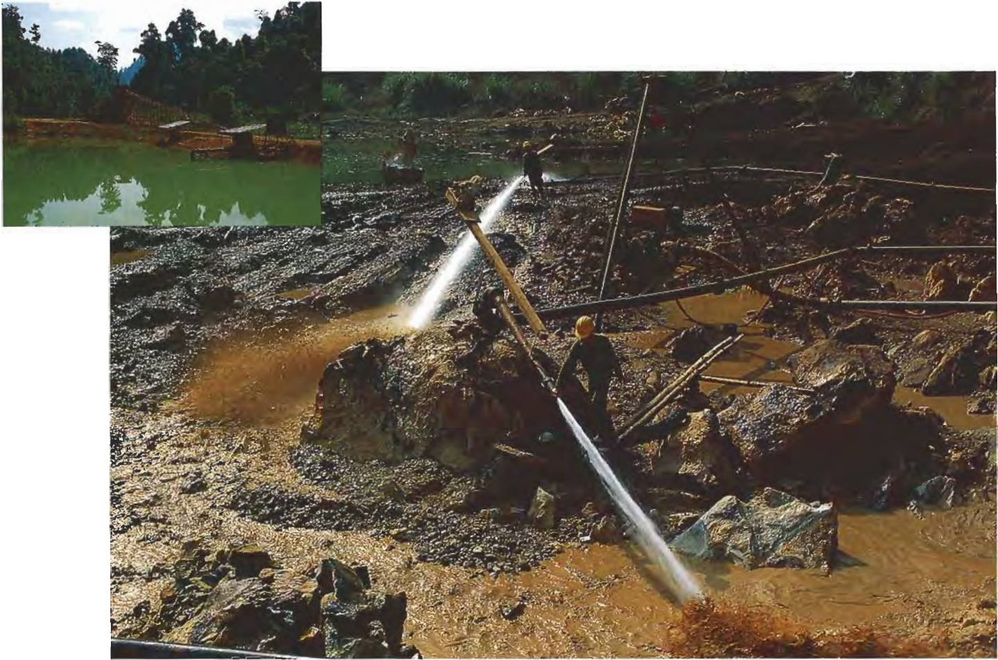
Figure 2. Khoan Thong I was the only deposit in Luc Yen being mined with heavy equipment during the authors' late-1992 visits. Here, high-pressure water cannons wash soil and gem-bearing gravels into a pit for subsequent processing. By November 1993 (inset), mining at Khoan Thong had almost ceased, and the original excavation had become an artificial lake not unlike the one at Mogok, Myanmar. Photos by Robert C. Kammerling.
