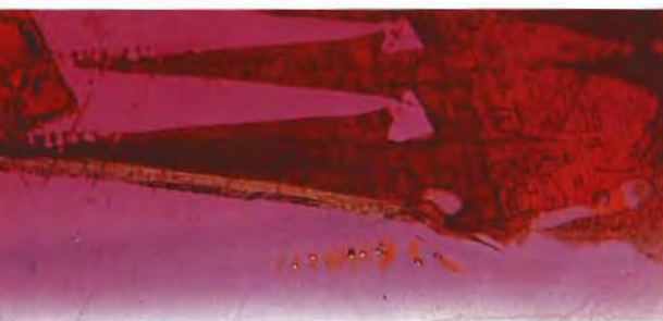
Figure 9. Purple to bluish purple color bands (like the one shown here in the lower part of the photo) were occasionally seen in tabular Douros synthetic ruby crystals, as were acute-angle purple to bluish purple triangular growth zones (like the one seen here in the lower left). A distinct iron/titanium component, in addition to the chromium component of ruby, is responsible for this color zoning. The inclusions shown here are flux. Magnified 10 \times .
