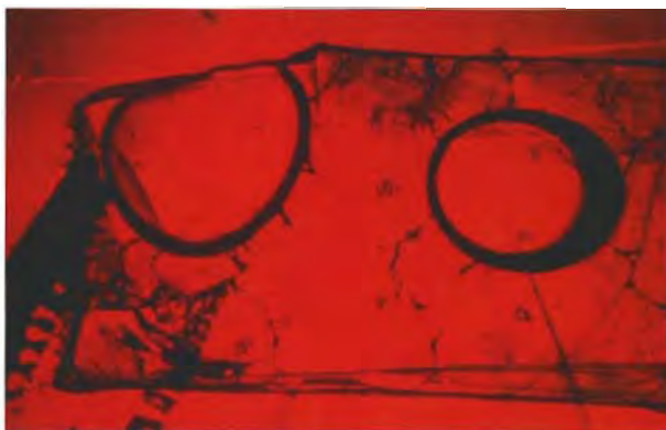
Figure 17. This large piece of flux in a Douros synthetic ruby has a distinctive mosaic pattern and contains two bubbles. The fine lines—or "crazing"—in the solid part of the inclusion help distinguish such inclusions from two-phase inclusions that might be seen in a natural ruby. Immersion, magnified 25×.
