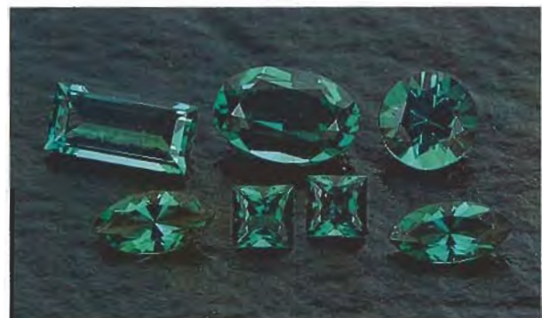
Figure 14. These faceted examples of "Swarogreen," a new glass imitation of emerald, range from 0.08 to 0.42 ct. Photo by Maha DeMaggio.
