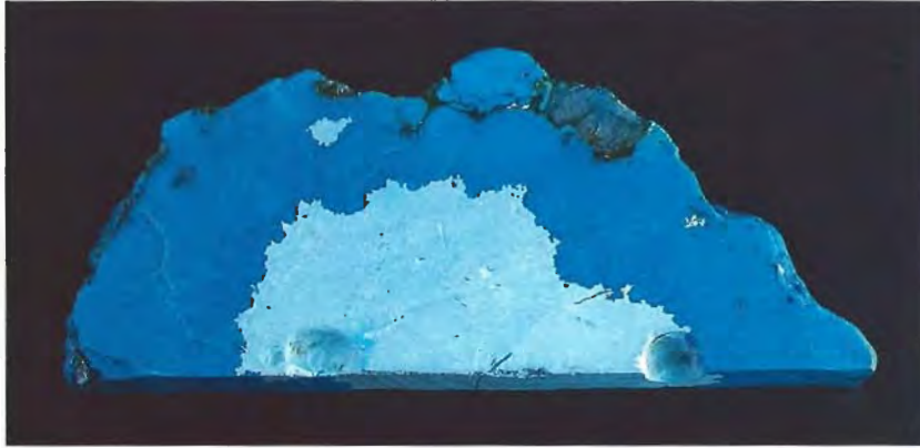
Figure 19. This 7.90 \times 3.23 \times 0.90 cm slab of dyed and impregnated natural turquoise clearly reveals the lighter blue color of the untreated material, in the center, where the treatment substance did not penetrate.
