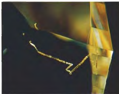
Figure 2. The squarish outline of the tube-like inclusions in this 4.03-ct fancy yellow diamond proved that they were etch channels. By comparison, the outlines of laser drill holes are typically round. Magnified 37×.
