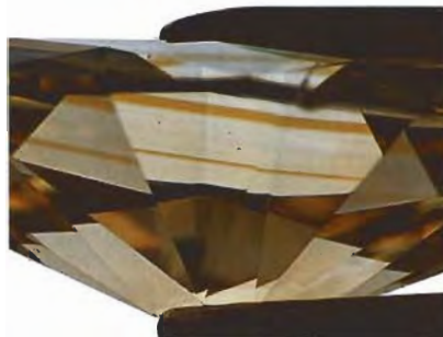
Figure 6. Parallel color banding is sharply defined in this 1.08-ct marquise brilliant-cut diamond, which measures 10.71 \times 5.25 \times 3.26 mm. Magnified 17 \times .
