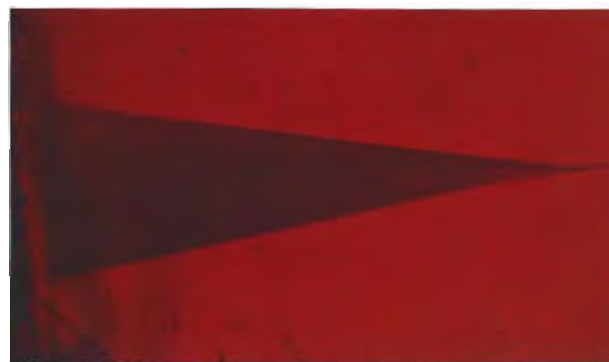
Figure 10. Acute-angle color zoning was also seen in rhombohedral Douros synthetic ruby crystals. Compare the appearance of the zone in this sample with that in the tabular Douros crystal in figure 9. Again, the bluish purple color is due to (Fe,Ti)-rich zones within the ruby crystal. Immersion, magnified 40 \times .
