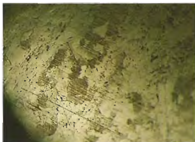
Figure 6. In reflected light, the bottom of this polymer-impregnated jadeite cabochon shows strong evidence of selective grain etching. Magnified 25 \times .
