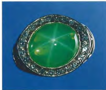
Figure 14. The unusual color in this synthetic star sapphire (about 14 \times 12 \times 5.90 mm) is probably due to \text{Co}^{3+} .
