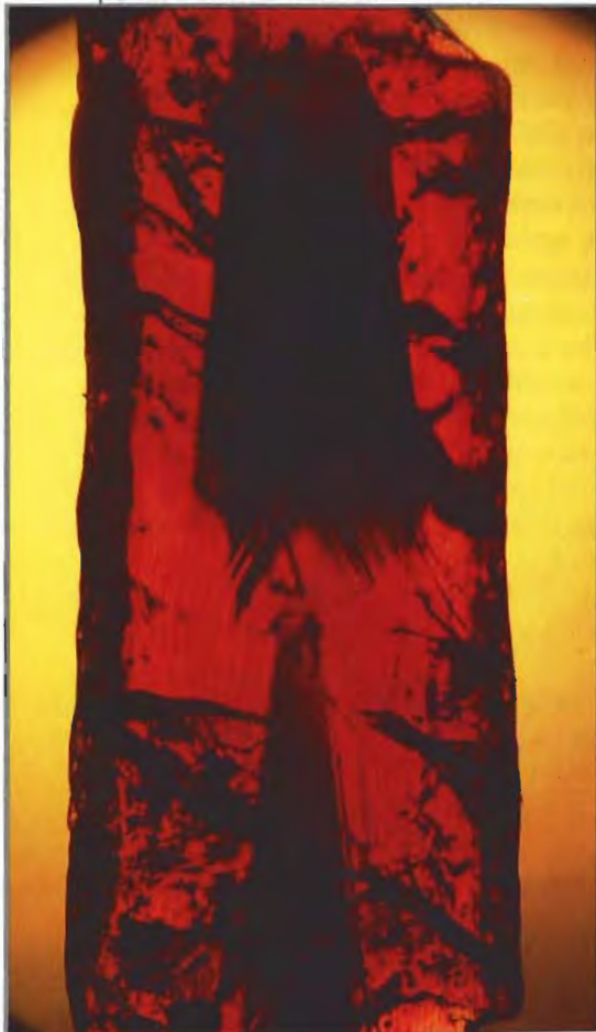
Figure B-1. This 10.5-mm-long untreated crystal, with two violet cores surrounded by red areas, illustrates the relationship between growth conditions and habit change typical of Mong Hsu rubies.
