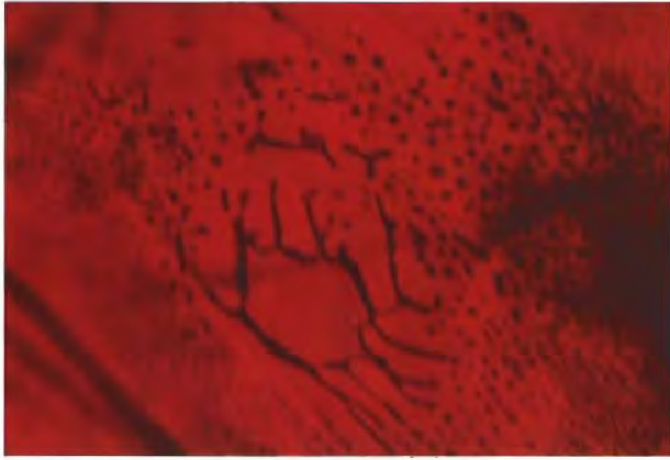
Figure 24. Healing feathers ("fingerprints")—actually interconnecting tubes and isolated dots of fluid inclusions—were commonly seen in both heat-treated (as here) and untreated Mong Hsu rubies. Immersion, magnified 60x.
