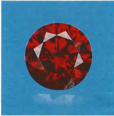
Figure 4. The dark red color of this 0.14-ct (about 3.23–3.27 × 2.07 mm) synthetic diamond is the result of treatment.
