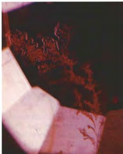
Figure 15. This dendrite in a 1.37-ct natural spinel could be confused with a flux inclusion in a synthetic spinel. Magnified 20 \times .
