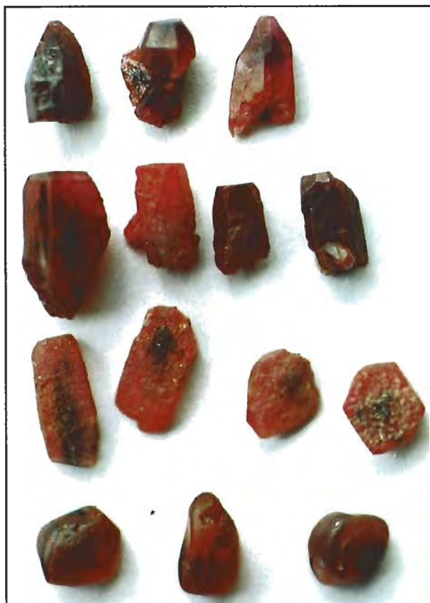
Figure 9. We selected these untreated pieces of Mong Hsu ruby rough from our study sample to illustrate some of the many different forms in which this material occurs. The first two rows are typical barrel-shaped, well-terminated crystals; the third row shows flat samples that are sometimes seen, which possibly formed in narrow veins; the waterworn crystals in the fourth row represent a minor proportion of the ruby lots. For an idea of size, note that the crystal on the far left in the upper row is approximately 8 mm long.
