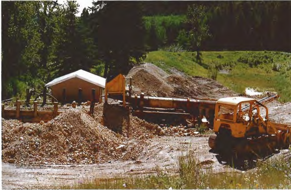
Figure 14. At the Vortex mine processing plant, ore is loaded into the yellow hopper, which feeds into the large rotating trommel. Heavy chains in the trommel help break down sapphire-bearing ore, which is then fed into a jig behind the bulldozer. Final clean-up of the sluice tray in the jig is done by hand. Photo by the author.
