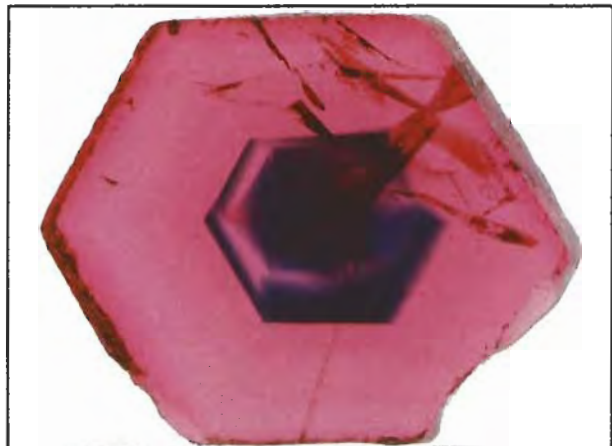
Figure 2. A distinctive feature of Mong Hsu ruby crystals is their deep violet (sapphire) core, which is surrounded by a red (ruby) rim. With heat treatment, the violet core becomes a deep red. This Mong Hsu ruby "thin section" is 5.3 mm wide; photo courtesy of John Emmett.
