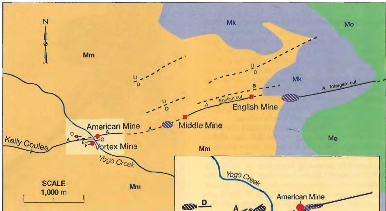
Figure 4. The Yogo sapphire deposit consists of at least six subparallel lamprophyre dikes, labeled by the author as "A", "B", "C", etc. All but the "B" (commonly called the "barren" dike) are known to be sapphire bearing. The vast majority of sapphire production at Yogo has been derived from the main A dike; it is this dike that is commonly referred to when the Yogo sapphire deposit is discussed. The inset provides detail on the area that is currently active. The dike system has intruded into limestone of the Mission Canyon formation (Mm) and shales of the younger Kibbey (Mk) and Otter (Mo) formations, probably along a pre-existing fault or fracture. Dahy (1988) mapped several faults paralleling the dike system to both the north and south (where upthrown side = U and downthrown side = D). Map modified from Dahy (1991).
