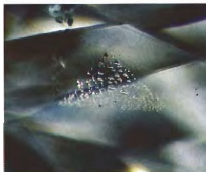
Figure 3. The triangular growth features in this diamond form a plane associated with the octahedral face of an enclosed phantom diamond crystal. Magnified 30 \times .
