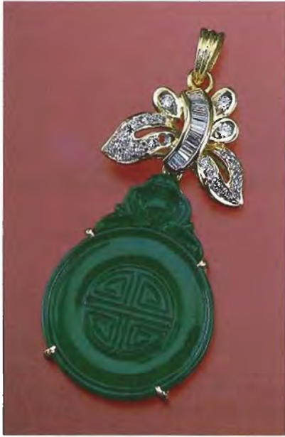
Figure 10. This 25.05 × 18.72 mm mounted carving proved to be an assemblage of jadeite jade and plastic.
