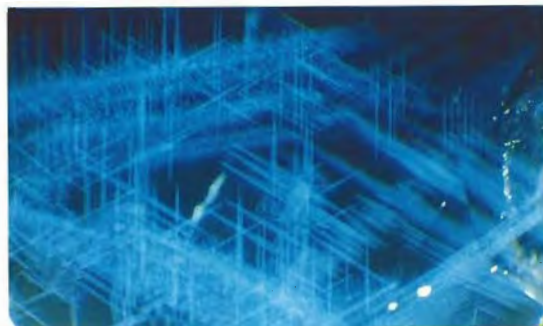
Figure 18. Some of the more distinctive inclusion features consisted of unique cross-hatch (left) to lath-like (right) cloud patterns, composed of individual whitish particles which resemble thin "blades" or very fine acicular crystals. Left: Darkfield illumination, magnified 15 \times ; photomicrograph by Dr. Eduard J. Gübelin. Right: Oblique fiber-optic illumination, magnified 25 \times .
