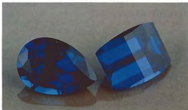
Figure 20. The Czochralski method was used to produce these two synthetic sapphires (1.64 and 1.76 ct). Photo by Maha DeMaggio.
