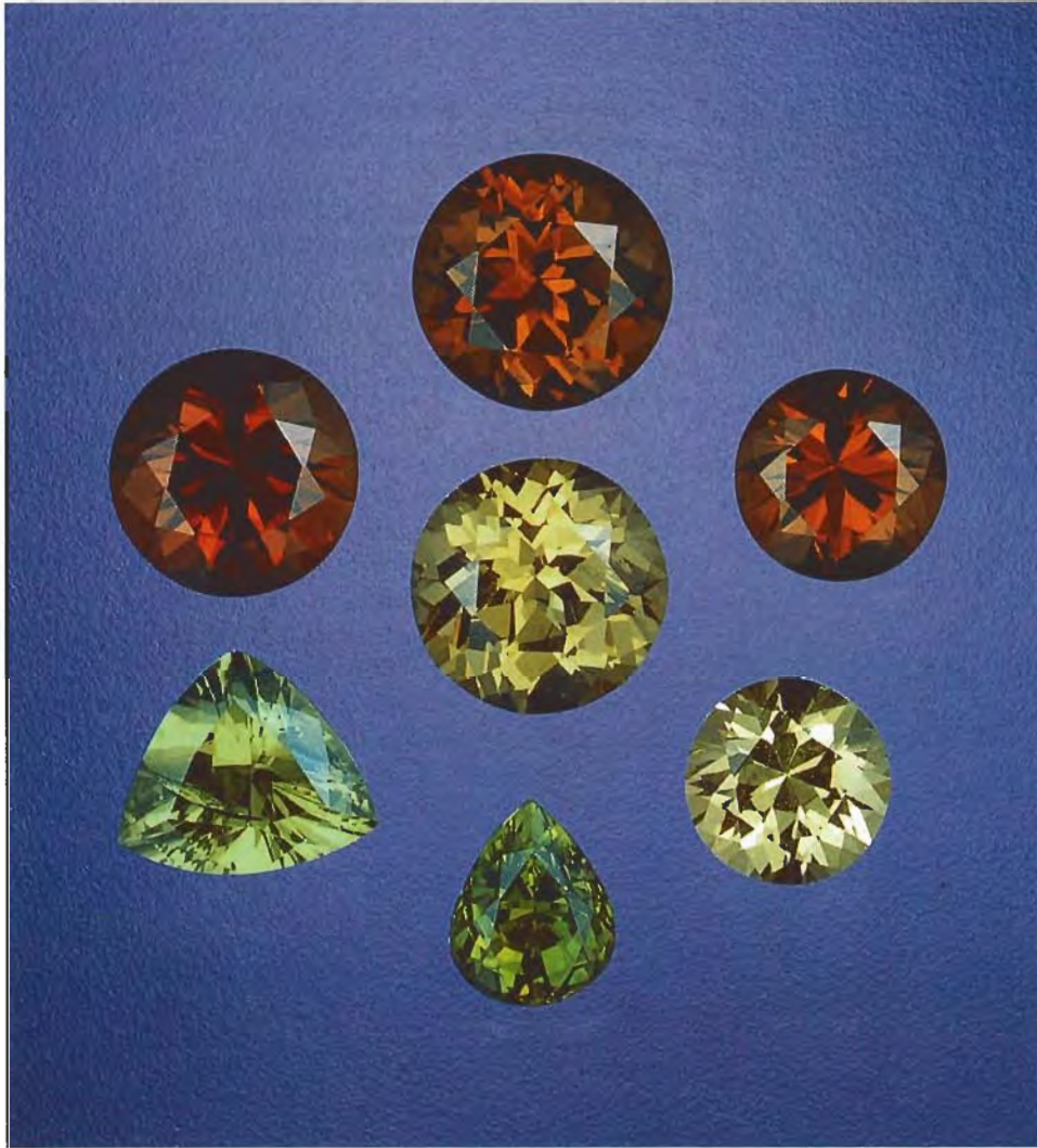
Figure 6. These seven faceted brown, yellow-green, and green grossular-andradite garnets from Mali (ranging from 0.85 to 2.39 ct) are part of the study sample. Stones courtesy of Pala Properties International and Thomas M. Schneider; photo © GIA and Tino Hammid.
