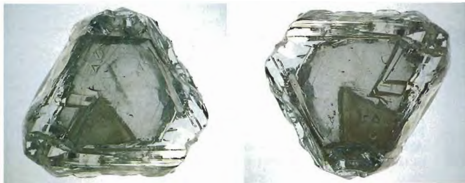
Figure 1. Note the movement of this triangular diamond inclusion in a large cavity when its host 1.09-ct macle is turned 180°. Photos by John I. Koivula.
