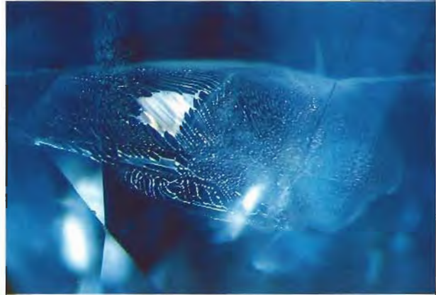
Figure 26. Healed fractures were common in the sapphires from southern Vietnam. Oblique fiber-optic illumination, magnified 35 \times .
