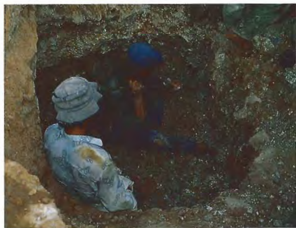
Figure 3. At Da Ban, most of the mining is done with simple hand tools, like the pick used by these miners to remove the potentially gem-bearing gravels. Photo by R. C. Kammerling.
