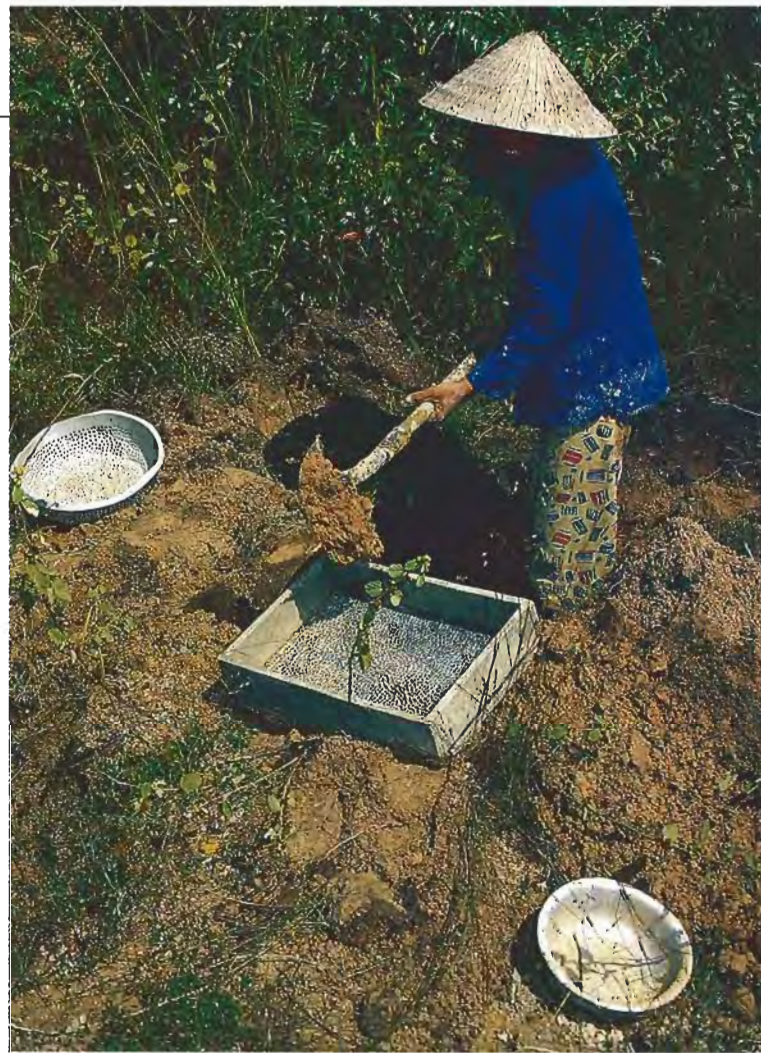
Figure 4. This miner throws gravel into a simple metal sieve for washing at Ma Lam. As at Da Ban, many miners work in the hot sun, shoveling dirt and gravels, and then carrying the heavy sieves to nearby ponds. Photo by R. C. Kammerling.
