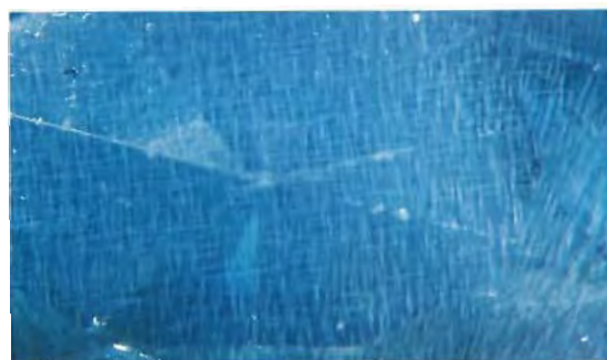
Figure 18. Some of the more distinctive inclusion features consisted of unique cross-hatch (left) to lath-like (right) cloud patterns, composed of individual whitish particles which resemble thin "blades" or very fine acicular crystals. Left: Darkfield illumination, magnified 15 \times ; photomicrograph by Dr. Eduard J. Gübelin. Right: Oblique fiber-optic illumination, magnified 25 \times .
