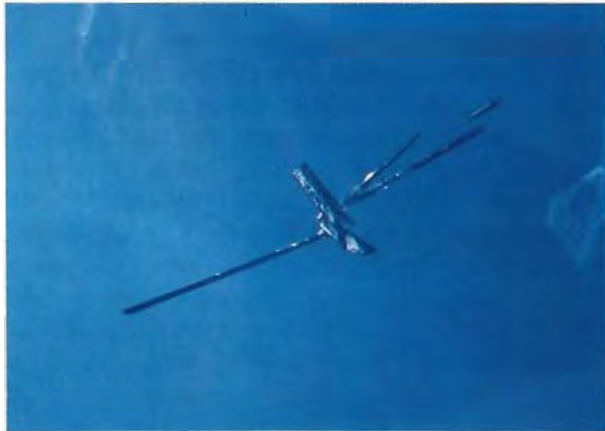
Figure 23. The southern Vietnam sapphires also contained groups of black-appearing acicular columbite crystals. The thinner "rods" displayed a rich red color along the edges when viewed with a pinpoint fiber-optic light source. Magnified 42 \times .
