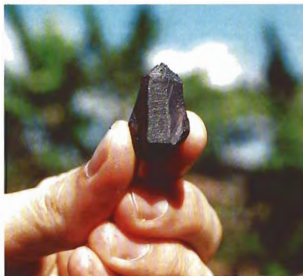
Figure 20. This rough "crystal" of purple GGG was misrepresented to a jeweler in Taunggyi, Myanmar, as a corundum gem from a new locality. Photo by Robert C. Kammerling.
