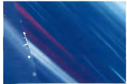
Figure 11. Red luminescence to intense transmitted light is confined to distinct bands, such as the one shown here, in this 19.45 ct blue sapphire. Magnified 20x.
