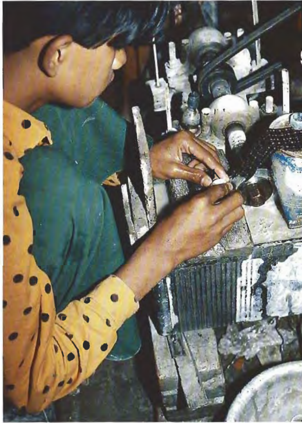
Figure 7. In a small lapidary shop in Mandalay, Myanmar, a worker saws a double ring blank in half to produce ring "preforms." Photo by Robert C. Kammerling.
