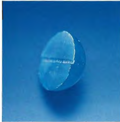
Figure 5. Once the stone in figure 4 was taken out of its setting, we realized that the "cabochon" was actually half a bead. Note the weak fluorescence of the adhesive to long-wave UV.
