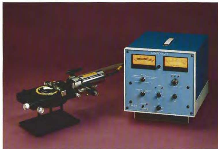
Figure 3. The Luminoscope, manufactured by Premier American Technologies Corp., consists of two parts: On the left is the vacuum chamber and electron "gun," and on the right is the power supply and control unit. Diamonds will emit visible cathodoluminescence when they are bombarded by the electron beam in the vacuum chamber. Photo courtesy of Premier American Technologies Corp., Bellefonte, Pennsylvania.
