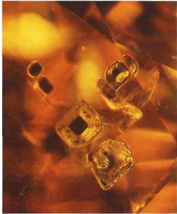
Figure A-1. A group of metallic inclusions is seen here under the table facet of a brownish yellow synthetic diamond. Although the square shape of the inclusions is somewhat unusual, their opaque appearance in transmitted light is very characteristic. Photomicrograph by John I. Koivula; magnified 25 \times .
