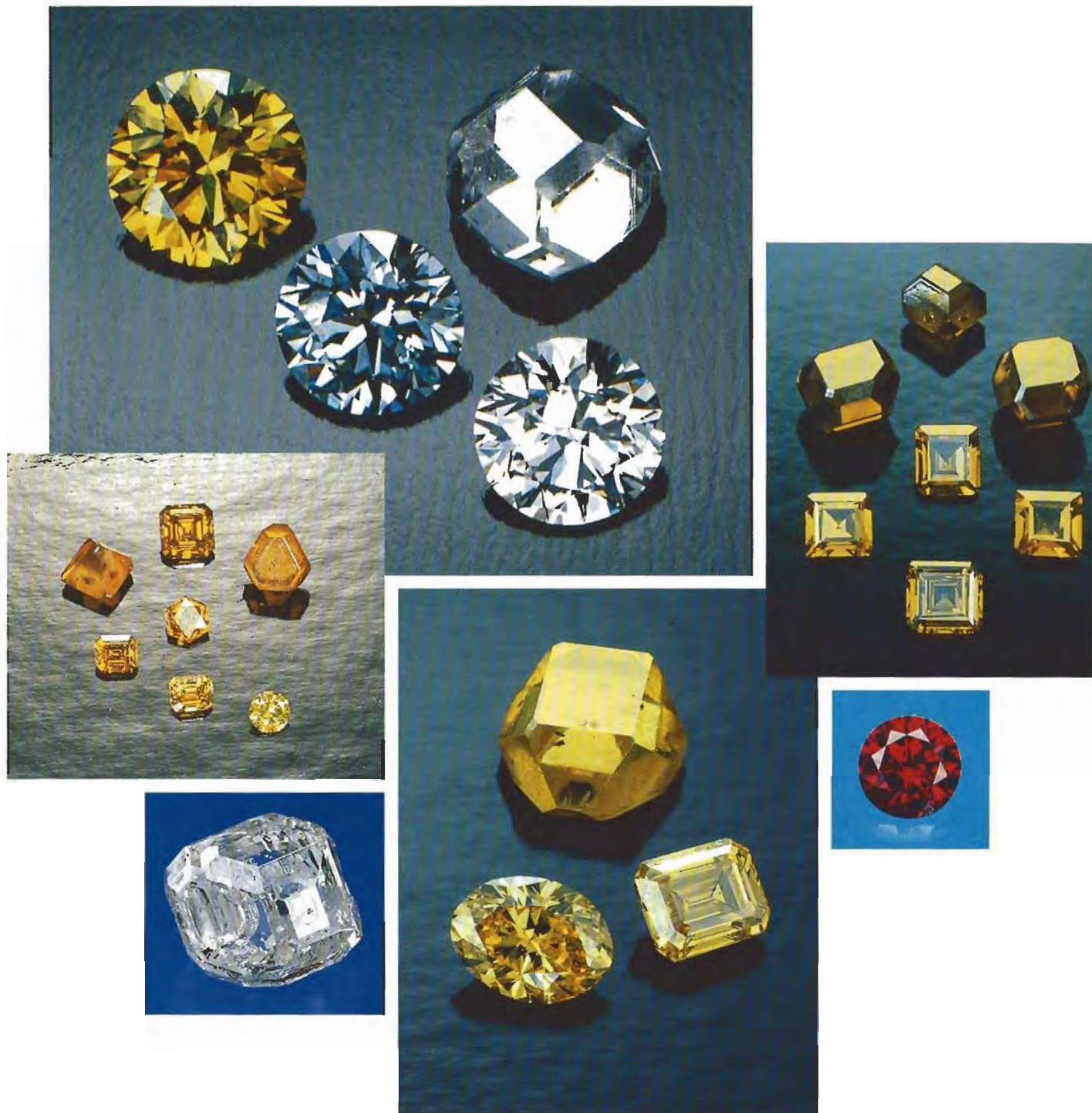
Figure 1. Shown here are some of the synthetic diamonds examined by GIA researchers to date (clockwise from top photo): (1) three faceted (0.39 ct yellow, 0.31 ct grayish blue, and 0.30 ct near-colorless) synthetic diamonds and one crystal (0.73 ct near-colorless) grown experimentally by General Electric; (2) three Sumitomo yellow crystals (top, 0.63–1.07 ct) and four yellow synthetic faceted stones (0.16–0.24 ct); (3) a 0.14 ct synthetic diamond with a dark red color caused by treatment; (4) De Beers experimental yellow synthetic diamonds—0.30 ct (left), 0.27 ct (right), and a 1.03 ct crystal (top); (5) a 0.42 ct near-colorless crystal produced in Russia; (6) two yellow Russian as-grown crystals (left, 0.78 ct; right, 0.88 ct), plus three as-grown (0.18–0.51 ct) and two treated (0.14–0.21 ct) faceted synthetic diamonds. Photos are by, again clockwise from top, Tino Hammid (first two), Shane F. McClure, Tino Hammid, Shane F. McClure, and Robert Weldon.
