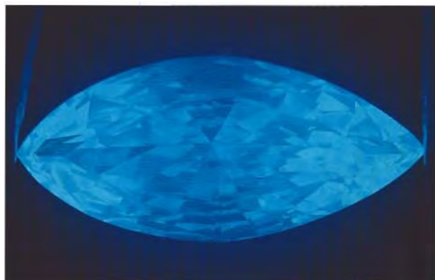
Figure 2. Natural diamonds, like the 0.69 ct near-colorless stone shown here on the left, typically fluoresce a relatively even blue to long-wave UV radiation. In contrast, synthetic diamonds, like this 0.13 ct yellow synthetic on the right, typically fluoresce yellowish green to short-wave UV radiation, with an uneven (cross-like) pattern (the blue color at the lower right is merely a reflection of the UV lamp). Photomicrographs by John I. Koivula; magnified 5× (left) and 15× (right).
