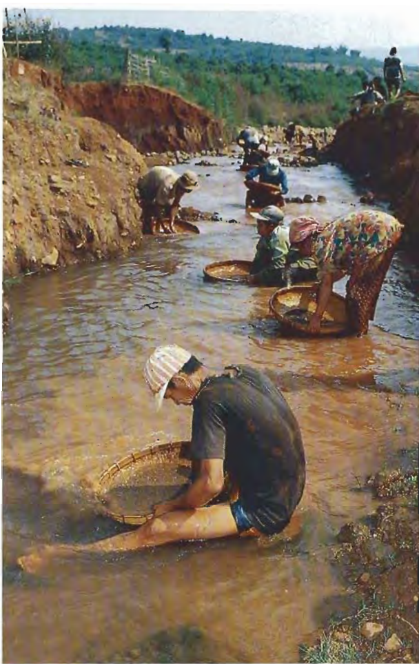
Figure 16. Soil and gravels, recovered from pits like that shown in figure 15, are washed for sapphires in a local stream. Photo by Robert C. Kammerling.
