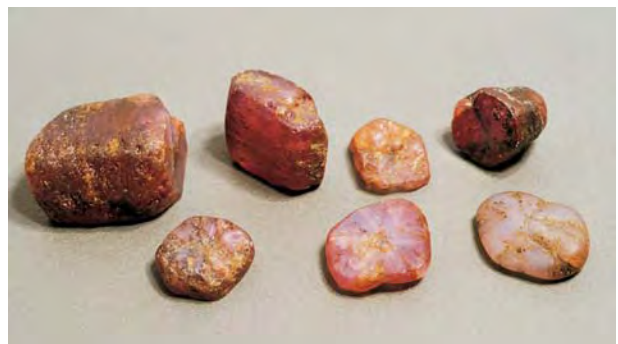
Figure 12. These “trapiche” rubies from Vietnam show tabular and barrel-shaped habits. The fixed “star” is formed by mica inclusions. Photo by H. A. Hänni.
