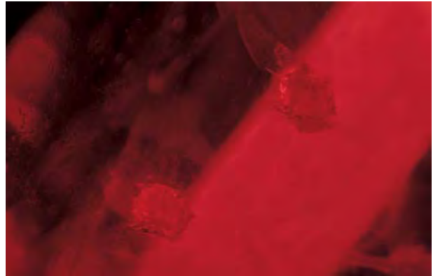
Figure 18. The smaller of the two rubies in figure 17 contained two melted-looking inclusions with numerous bubbles. Photomicrograph by John I. Koivula; magnified 20×.
