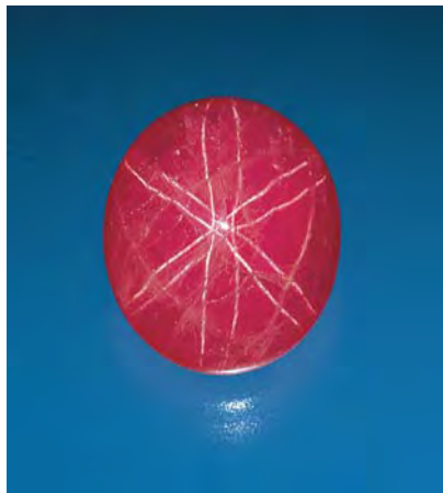
Figure 12. The true double star in this 8.19 ct ruby is caused by differences in the orientation of rutile “silk” across pervasive twin planes.
