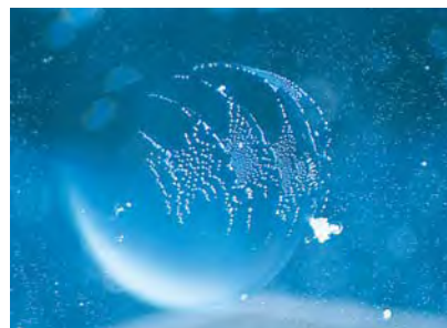
Figure 9. A small droplet of glass encapsulates a fingerprint-like formation of gas bubbles that is sandwiched between the blue and colorless layers in the piece of faceted glass shown in figure 8. Magnified 15×.
