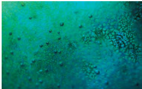
Figure 15. When the nacre was examined with an intense fiber-optic light transmitted through the crown, numerous gas bubbles in the polymer were visible through the nacre of five samples. Note that the blue polymer, illuminated through the nacre, appeared green in some. Sample courtesy of Empress Abalone Ltd.; photomicrograph by John I. Koivula, magnified 40×.
