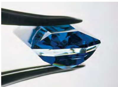
Figure 8. Blue and colorless layers are readily apparent in this 4.28 ct faceted piece of manufactured glass when it is viewed along the girdle plane. In this view, the blue color in the pavilion is reflected into a large portion of the crown.
