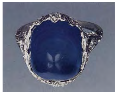
Figure 16. This ring appears to have been manufactured in the early part of this century. The Verneuil synthetic sapphire in the center shows eye-visible concentric circles of color banding.
