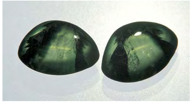
Figure 8. Both of these free-form double cabochons, which were cut from a single trapiche emerald crystal, show chatoyancy. These 2.05 and 2.15 ct samples measure 10.79 × 7.78 × 3.32 and 10.98 × 8.01 × 3.33 mm, respectively. Courtesy of Collectors; photo by Maha DeMaggio.
