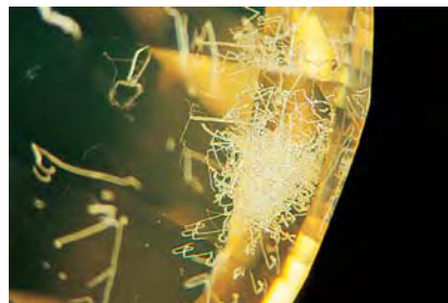
Figure 5. This dense tangle of natural etch channels was typical of the numerous etch features observed in a 25.02 ct brownish yellow round brilliant diamond. Magnified 17 \times .
