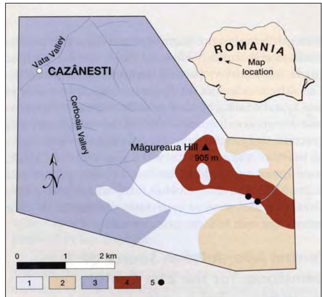
This geologic map of the Vata area (after Cioflica, 1960) shows the occurrence of the gem-quality vesuvianite and grossular. Key: 1—Upper Jurassic limestones; 2—Lower Cretaceous clays and sandstones; 3—Mesozoic ophiolites; 4—Upper Cretaceous intrusives; 5—Vesuvianite + grossular + wollastonite + gehlenite + Ti-andradite (melanite) occurrences.
