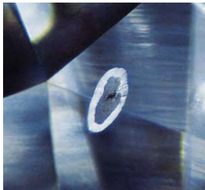
Figure 14. In most of the 103 samples that had solid inclusions surrounded by a stress crack, a black inner area (graphite) was surrounded by a brighter halo of outward radiating cracks (left; also evident here is the banded internal graining seen in a number of the GE POL diamonds). In some instances, there were several areas of graphite (right). Photomicrographs by John I. Koivula; magnified 40 \times .
