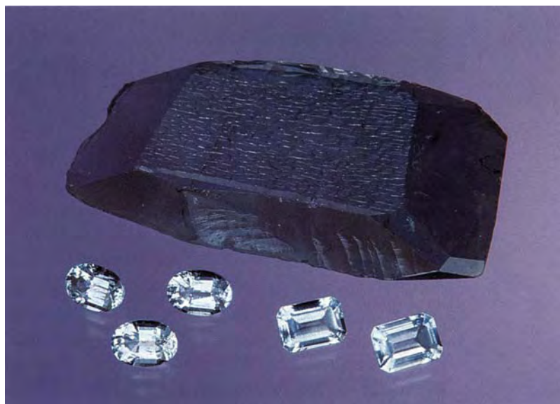
Figure 2. One of the newest synthetics on the market is hydrothermally grown synthetic aquamarine. The cut samples average approximately 1 ct. Photo by Maha DeMaggio.
