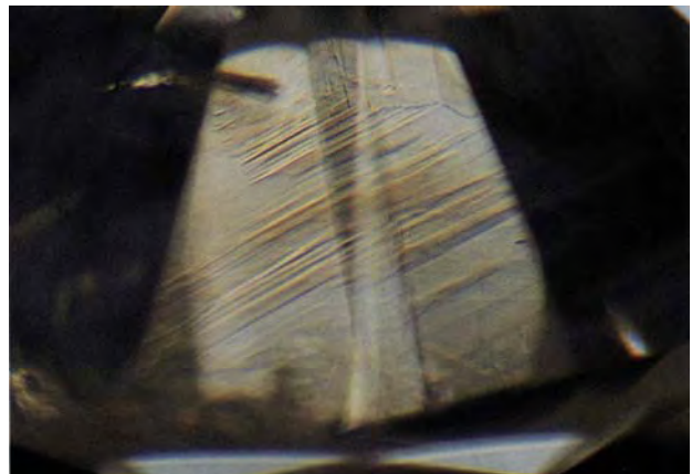
Figure 9. Also observed was brown graining, often in a parallel banded pattern. Photomicrograph by Shane F. McClure; magnified 40 \times .
