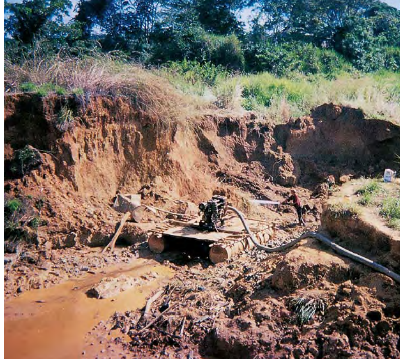
Figure 1. Water cannons are used to mine diamonds near the Quebrada River in the Guaniamo region of Venezuela. Photo by Ric Taylor.
