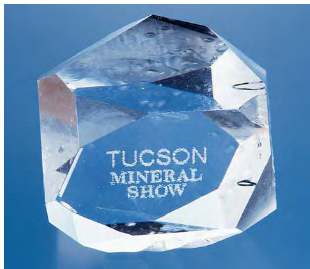
Figure 27. The words in this 42-mm-long synthetic quartz crystal were inscribed completely internally by a laser technique. Photo by Maha Tannous.
