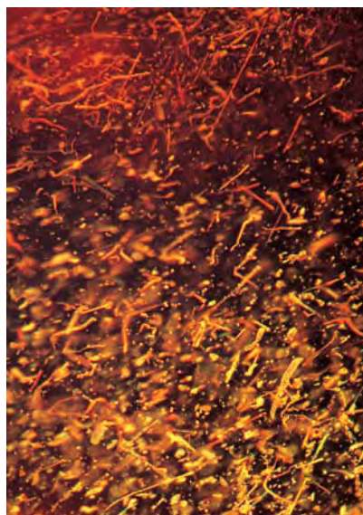
Figure 13. The numerous skeletal inclusions in this sapphire appeared to be responsible for at least part of the bodycolor of their host. Magnified 40x.
