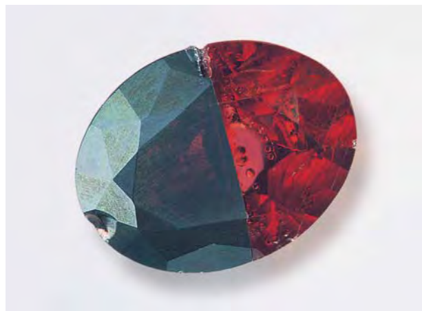
Figure 22. The heat-treated portion of this 5.60 ct almandine-spessartine garnet (left) developed a dark gray metallic coating that was identified as hematite. Photo by Maha Tannous.
