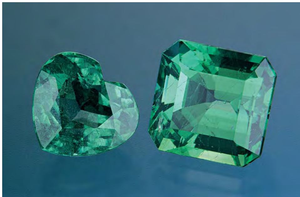
Figure 7. Degree of enhancement is only one factor that may affect a stone's value. The emerald on the left has many inclusions that are highly visible, yet it merits only a "minor" enhancement call because it has relatively few filled surface-reaching fissures. The eye-clean stone on the right appears to be of very high quality. However, the clarity enhancement is masking several large fractures. The emerald would look much worse if it were not filled, so it deserves a "significant" classification. Photo by Maha Tannous.
