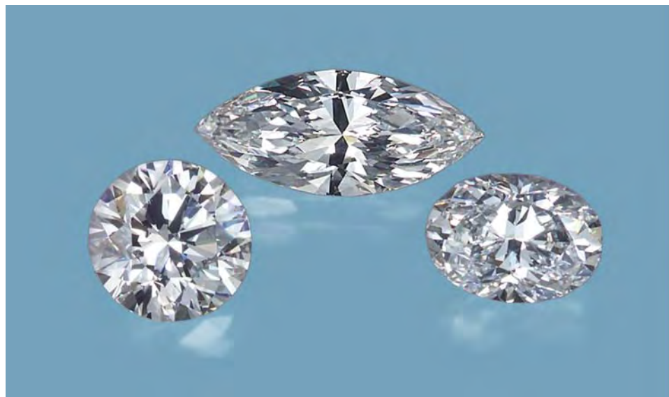
Figure 1. These three GE POL diamonds (4.11–5.34 ct) were all decolorized by a high-pressure, high-temperature process developed by General Electric. Photo by Elizabeth Schrader.
