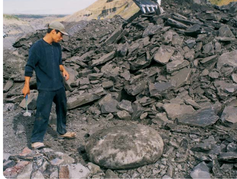
Figure 6. A Korite employee inspects a recently uncovered ironstone concretion from the K Zone (see text) of the Kormos mine. The disk shape of this concretion is an indication that an ammonite—and therefore Ammolite—may be found within. Photo by Art Barnson, Barnson Photography.
