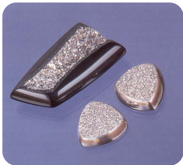
Figure 24. The glittering appearance of these pieces results from a thin coating of platinum that has been applied over drusy gem materials. The two smaller pieces measure approximately 11.5 mm in maximum dimension. Photo by Maha Tannous.
