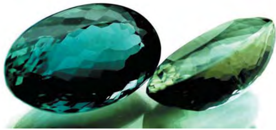
Figure 4. Both of these beryls (30.67 ct and 23.64 ct) show a strong green-blue color when viewed face-up parallel to the optic axis (left). Strong pleochroism is evident when viewed from the side, where a greenish yellow color is seen perpendicular to the optic axis (right).
