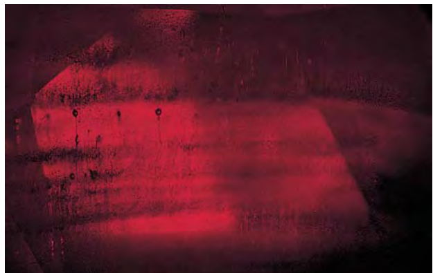
Figure 40. When examined with a microscope, the streaks of "silk" were revealed to be slightly curved zones of gas bubbles, which proved the ruby was synthetic. Photomicrograph by Jaroslav Hyrsl; field of view is 1.7 mm.
