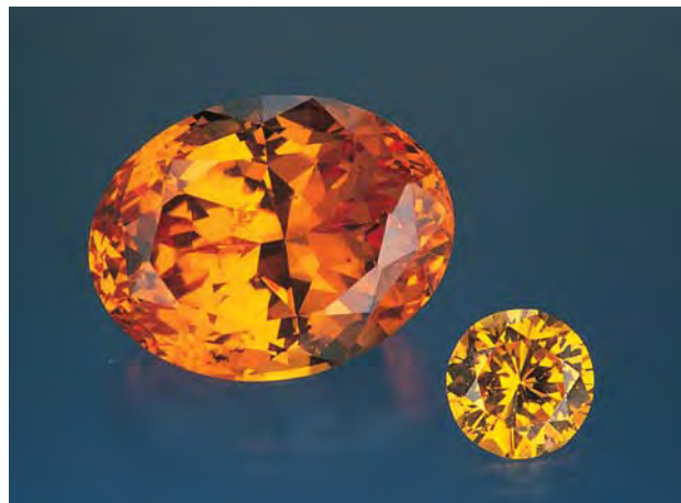
Figure 36. These two faceted samples of the synthetic material “langasite” ( \text{La}_3\text{Ga}_5\text{SiO}_{14} ) were grown in Russia by the Czochralski method. They weigh 56.80 and 4.59 ct. Photo by Maha Tannous.
