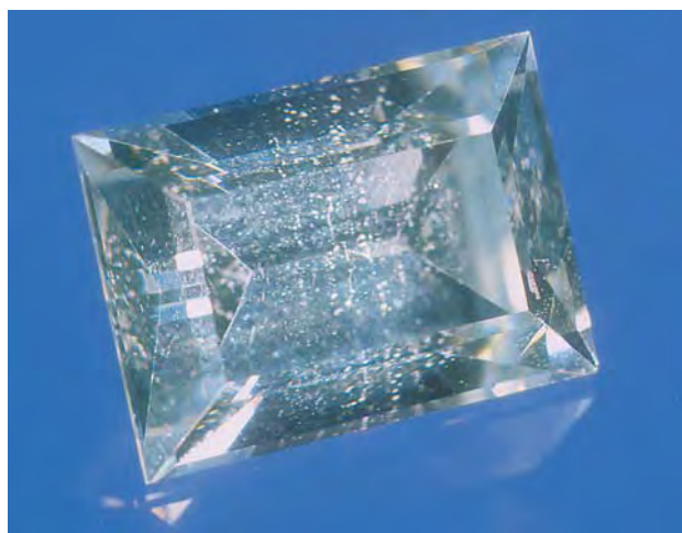
Figure 37. This laboratory-grown 5.45 ct rectangular step cut ( 11.1 \times 6.9 \times 5.1 mm) was represented as “langasite.” Chemical analysis of the sample revealed a composition that is consistent with a theoretical formula of \text{SrLaGa}_3\text{O}_7 , which differs from that of langasite, \text{La}_3\text{Ga}_5\text{SiO}_{14} . Photo by Alain Cossard.
