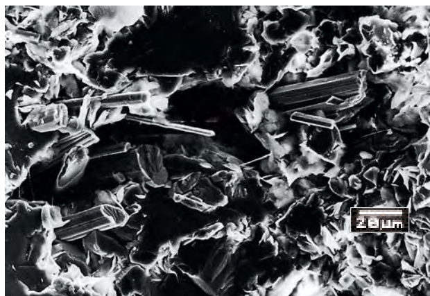
Figure 31. This scanning electron micrograph of a broken piece of "Spider" quartz from Madagascar shows the fine needle-like inclusions that were identified as hollandite.
