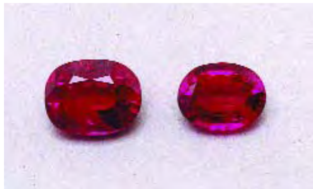
Figure 30. These two flux-grown synthetic rubies (7.61 and 4.49 ct) had an unusual combination of properties, including trace-element contents that have not been recorded previously. Photo by H. Hänni.
