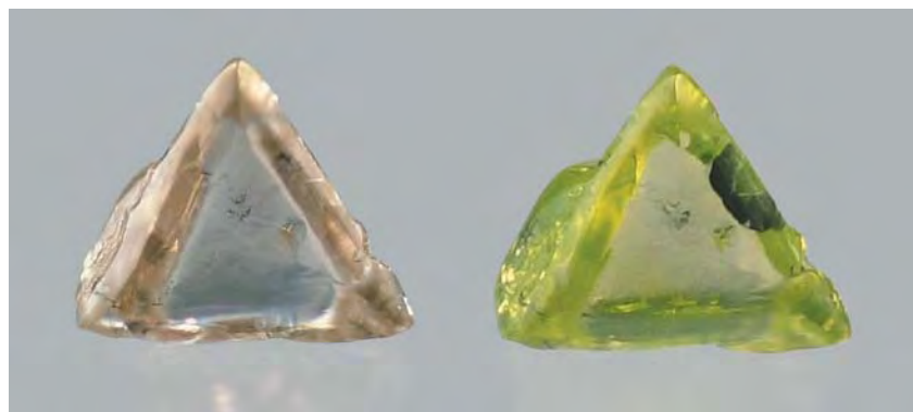
Figure 2. After HPHT treatment, this type Ia diamond (1.07 ct) changed from brown to green-yellow.
