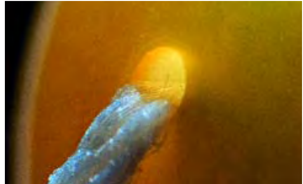
Figure 3. In many of the cultured pearls, the color appeared to be concentrated near the surface when viewed down the drill hole. Such concentrations of color in pearls are good indicators of treatment. Photomicrograph by John Koivula; magnified 5 \times .
