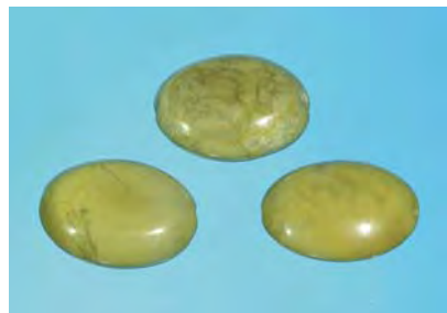
Figure 14. Advanced testing revealed that these three beads (each approximately 14.00 \times 10.00 \times 5.00 mm) were fashioned from the rare gem material schlossmacherite.
