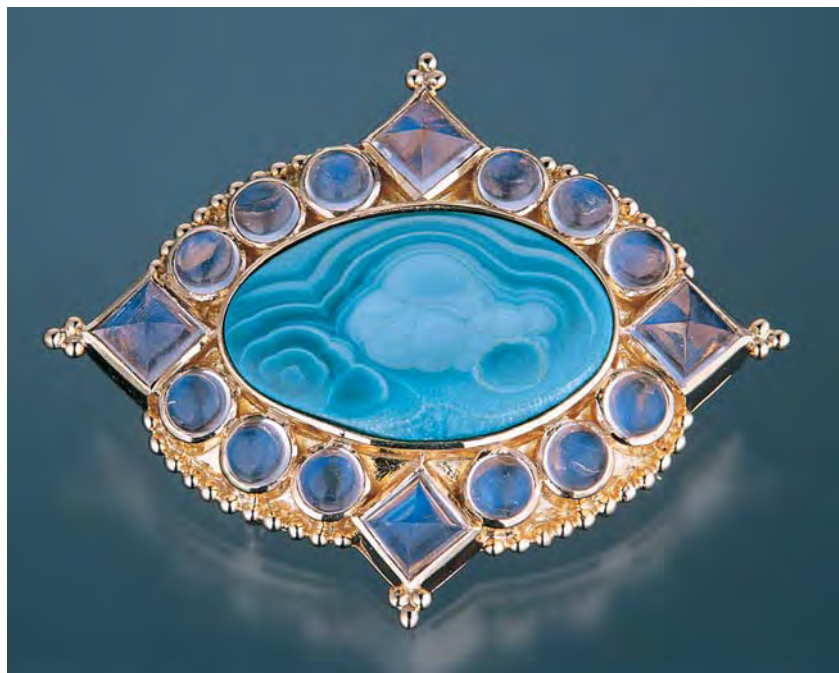
Figure 1. Advanced testing proved that the unusual center stone (29.50 × 18.10 mm) in this combination brooch and pendant was aurichalcite.
