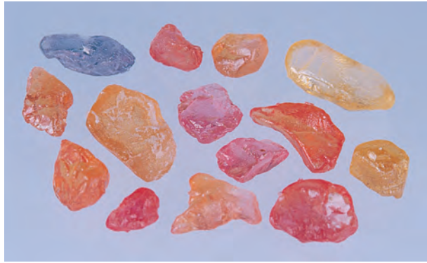
Figure 24. Experiments 1–4 in this study were able to reproduce every color and color layer that we had observed in the Be-diffused samples processed in Thailand. Some of those colors are shown by these corundum samples (0.4–2.1 ct). Photo by Maha Tannous.
