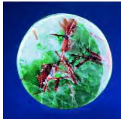
Figure 9. This 87.84 ct polished disk of Guatemalan jade contains reddish brown inclusions of lawsonite.
