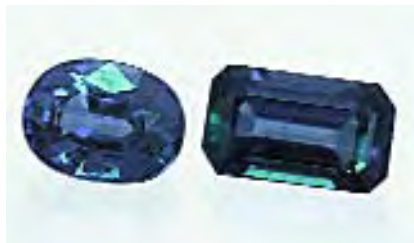
Figure 12. These sapphire/synthetic sapphire doublets (1.73 and 2.29 ct) showed a change-of-color from greenish blue in daylight-equivalent illumination (left) to reddish purple in incandescent light (right). The color change comes solely from the synthetic color-change sapphires that form the pavilions.
