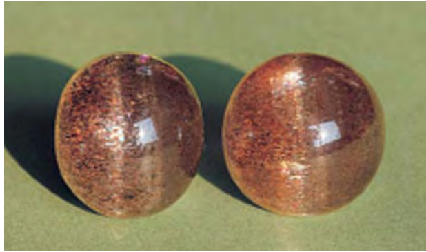
Figure 4. These cat's-eye beryl cabochons (24.78 and 23.67 ct) were purchased as quartz in Brazil. Photo by Jaroslav Hyrsl.
