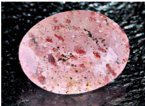
Figure 25. This 7.28 ct faceted rose quartz from Rakwana, Sri Lanka, hosts inclusions of spessartine and ilmenite. Photo by Maha Tannous.
