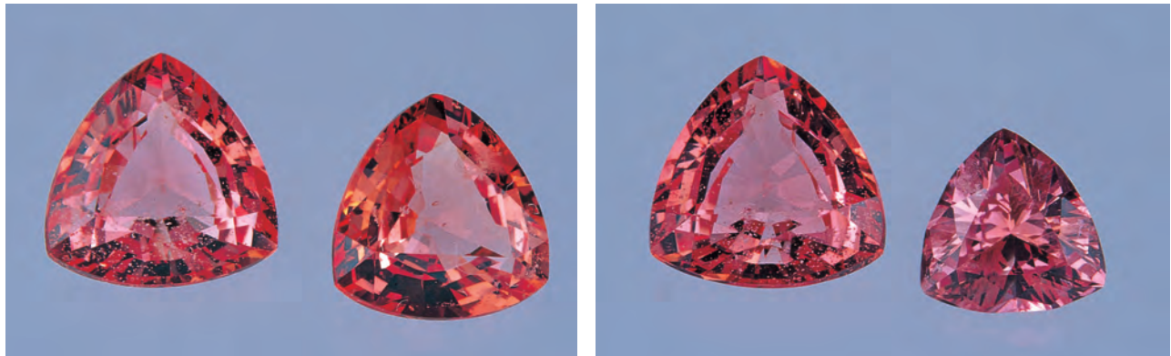
Figure 58. To illustrate the consequences of recutting incompletely Be-diffused stones, we took one of these two closely matched treated sapphires and had it recut as if it had been chipped and needed significant repair. The 0.71 ct stone on the right side of the pair was recut to 0.40 ct, and clearly has lost most of its orange component. Photos by Maha Tannous.
