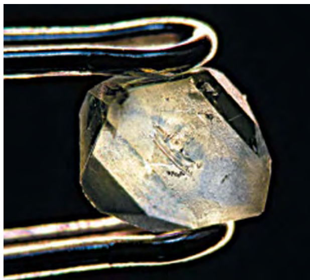
Figure 28. This 0.33 ct bicolored synthetic diamond crystal exhibits both blue and yellow zones. Photo by T. Hainschwang.
