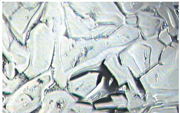
Figure 47. Blocky synthetic overgrowth produced during the Be-diffusion process was still present on the surface of some treated stones, even after repolishing. Photomicrograph by Ken Scarratt; transmitted light, magnified 30 \times .
