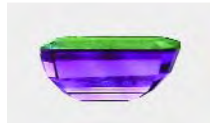
Figure 13. In profile, with diffused transmitted light, both parts of the doublet become evident, as do the curved color bands in the synthetic color-change sapphire pavilion.
