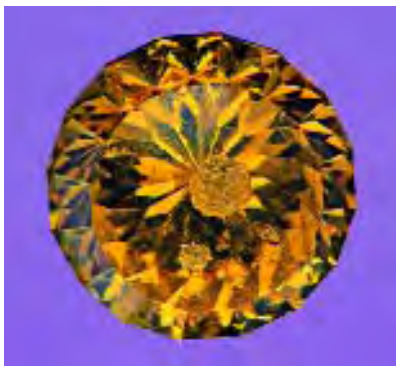
Figure 7. Two spherical inclusions, a “planet” and its “moon,” highlight the interior of this 27.73 ct faceted piece of manufactured glass.
