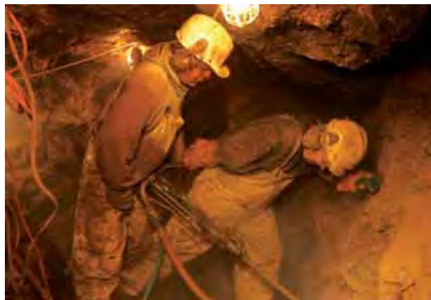
Figure 19. Possible extensions of the mineralization were explored by drilling a few carefully placed holes to depths up to 2 m. The drill is powered by compressed air and the bit is cooled by water, so even a few minutes of drilling produces a fine mist. Photo by B. M. Laurs.
