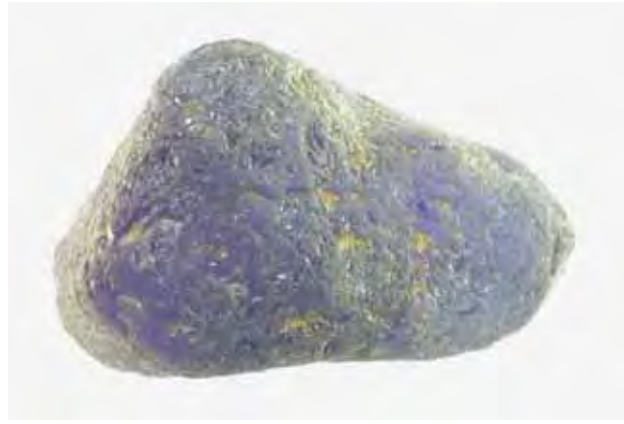
Figure 29. Though presenting a convincing appearance as a pebble of sapphire or tanzanite, this sample (34 × 21 × 20 mm) proved to be manufactured from cubic zirconia. Photo by Min Htut.
