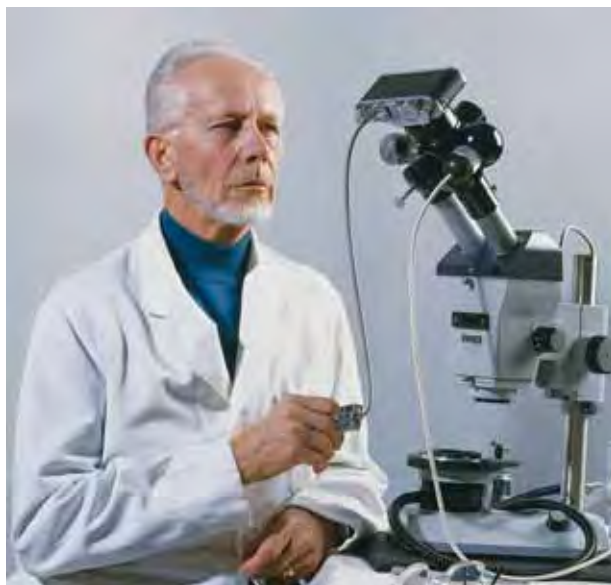
Figure 8. Throughout his career, Dr. Gübelin continuously refined his photomicrographic techniques. Here he is shown taking a photomicrograph with his Zeiss SV8 microscope with custom darkfield illumination.
