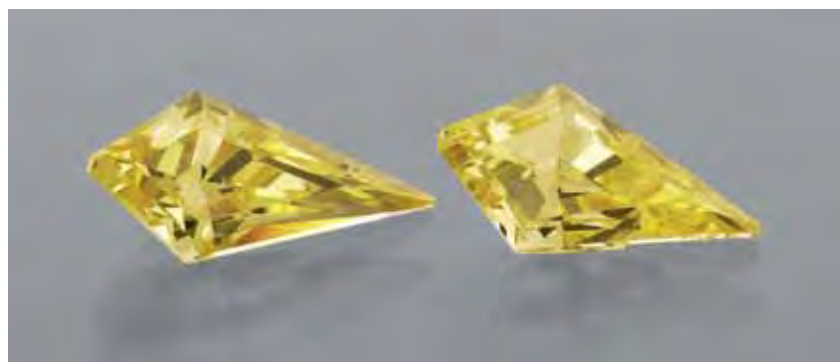
Figure 1. These two yellow samples of cubic zirconia (11.30 × 5.50 × 3.72 and 10.54 × 5.57 × 3.71 mm) could be mistaken for irradiated and annealed cape diamonds if a gemologist relied on their visible spectra to identify them.
