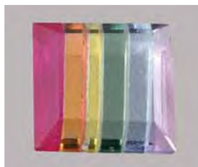
Figure 1. This unusual specimen was assembled from slices of synthetic ruby, synthetic quartz, and synthetic spinel.
