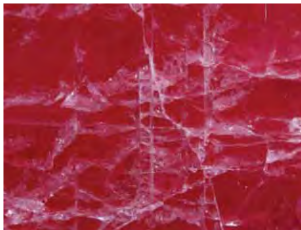
Figure 25. Ammonia, bleach, and even concentrated lemon juice damaged the lead-glass filler at the very surface, producing the whitish areas shown here. Photomicrograph by C. P. Smith; magnified 32×.
