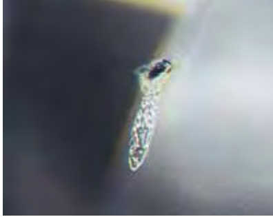
Figure 3. This fingerprint-like inclusion extends from a graphitized crystal in a colorless diamond that was recently proved to have been HPHT treated. Magnified 45×.
