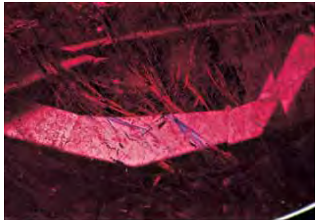
Figure 8. In some of the samples, the flash effect was very strong and an orange flash could also be seen. Here, the blue is quite strong in brightfield illumination, and the orange flash is easily seen in darkfield. Photomicrograph by S. F. McClure; magnified 10 \times .
