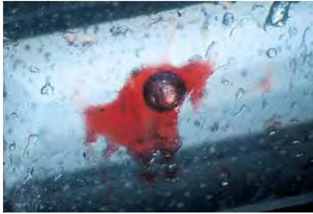
Figure 18. The unusual two-phase orange fluid inclusions in this quartz from Bahia, Brazil, are situated in two different growth zones, suggesting that they are primary inclusions and not the result of healed fractures. Photomicrograph by J. I. Koivula for microWorld of Gems ; magnified 10 \times .
