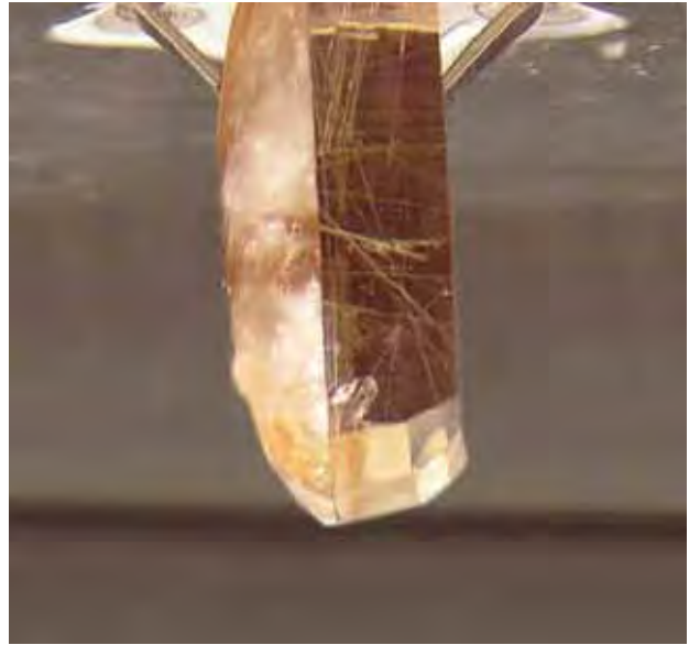
Figure 33. When this cabochon (20 mm in diameter) was viewed from the side in immersion, its assembled nature was readily apparent. This doublet consists of a layer of rutilated quartz with a backing of transparent quartz that contains little or no rutile. Photo by M. Macri.
