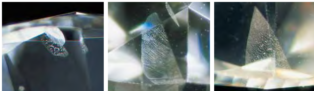
Figure 2. Fingerprint-like inclusions such as these have been reported in several colorless to near-colorless diamonds known to have been HPHT treated (from figure 10 in T. M. Moses et al., Fall 1999 Gems & Gemology , pp. 14–22). From left to right, magnified 32×, 18×, and 13×.
