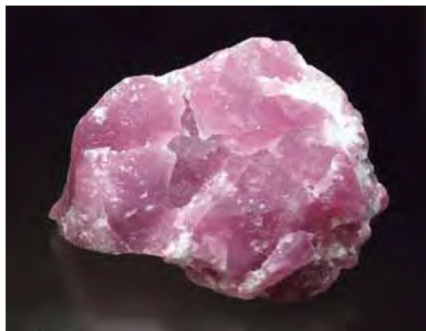
Figure 8. This aggregate of fine-grained muscovite (about 7 cm wide) was represented as rose quartz in Minas Gerais, Brazil. Photo by J. Hyršl.
