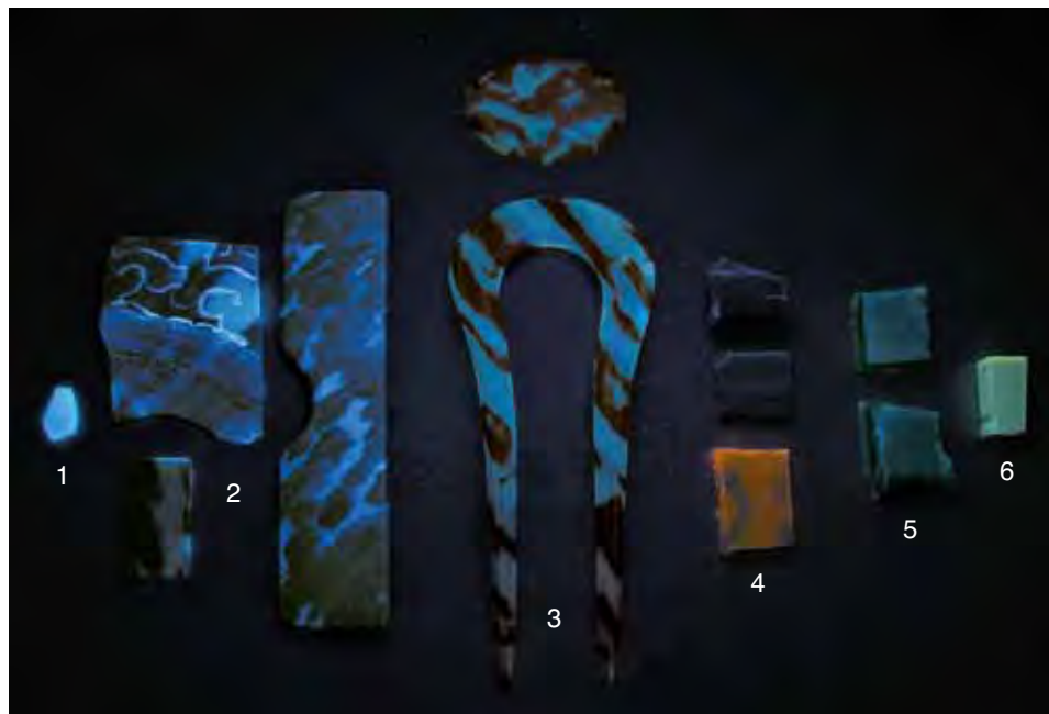
Figure 6. When exposed to long-wave UV radiation, the fluorescence reactions of the materials in figure 3 are quite distinct despite their similarities in normal light. As seen here, tortoise shell's chalky blue-white reaction usually can allow easy separation from imitations. From left: horn (1), tortoise shell (2), cellulose nitrate (3), cellulose acetate (4), polyester (5), and casein formaldehyde (6). Photo by T. Hainschwang.
