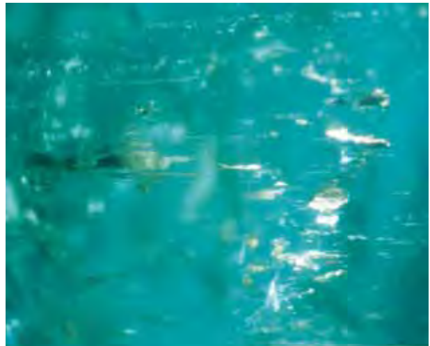
Figure 13. These brownish yellow-appearing metallic inclusions in Nigerian tourmaline were identified as native copper by LA-ICP-MS. The copper platelets are oriented parallel to the c -axis of the tourmaline. Photomicrograph by A. Abduriyim; magnified 60 \times .
