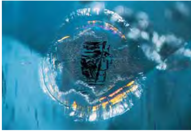
Figure 16. Framed by a thin ovoid tension fracture, this unusually large 2.1 mm skeletal ilmenite dendrite looks like a rather curious form of ancient cuneiform writing. Photomicrograph by J. I. Koivula for microWorld of Gems .
