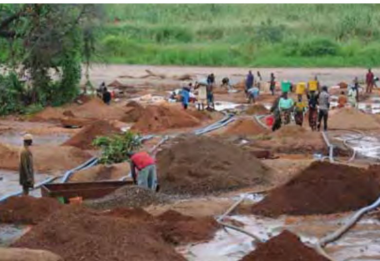
Figure 5. The gem-bearing soil is washed using water from Mtindiri River. The miners dig pits in the riverbed to make small reservoirs, and the water is pumped through a network of hoses to the washing screens. Photo by V. Pardieu/GGL.
