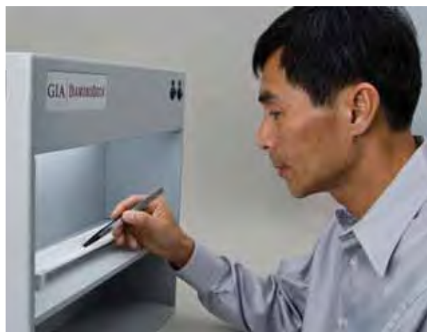
Figure 11. A standard “0/45” viewing geometry is used when color grading D-to-Z diamonds. The light source is above the tray at approximately “0” degrees, and the diamond is observed from a position approximately 12–15 in. (30–37.5 cm) away at an angle about 45° from the stone.
