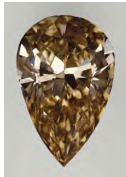
Figure 1. This 3+ ct Fancy Dark brown-yellow diamond was found to be distinctly type zoned (IIa and IIb).
