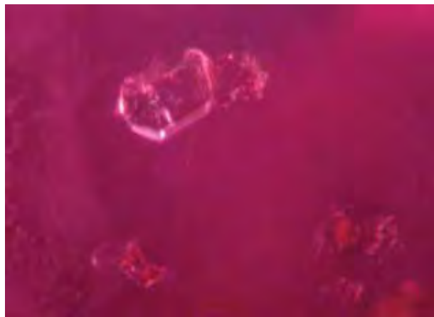
Figure 29. Colorless transparent apatite crystals were seen in only two Winza rubies. Photomicrograph by V. Pardieu/GGL; magnified 40×.
