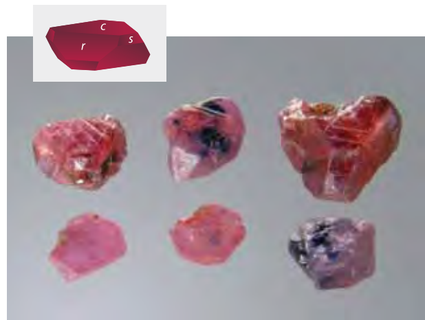
Figure 11. Several of the ruby and sapphire crystals examined (here, up to 8 \times 10 mm) had positive rhombohedral faces, or both positive and negative rhombohedral forms ( r and s , respectively). Depending on the size of the basal pinacoid c , a platy habit may result. Photo by K. Schmetzer.
