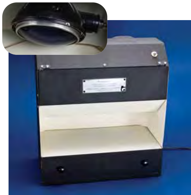
Figure 4. The GIA Diamolite was introduced to AGS members in 1941 and, for the first time, offered jewelers a controlled lighting and viewing environment for comparing "master" diamonds to other diamonds. The Diamolite measured 13\frac{3}{4} in. high \times 12 in. wide \times 6 in. deep (34.4 \times 30 \times 15 cm) and housed an incandescent bulb with a blue filter (inset) designed to make the light output better simulate daylight. Photos by Robert Weldon.
