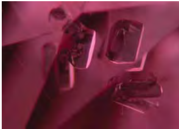
Figure 27. Well-developed prismatic amphibole crystals are common in Winza corundum. The amphiboles do not show any preferred orientation in the corundum host; they can be considered as protogenetic inclusions. Photomicrograph by V. Pardieu/GGL; magnified 40×.
