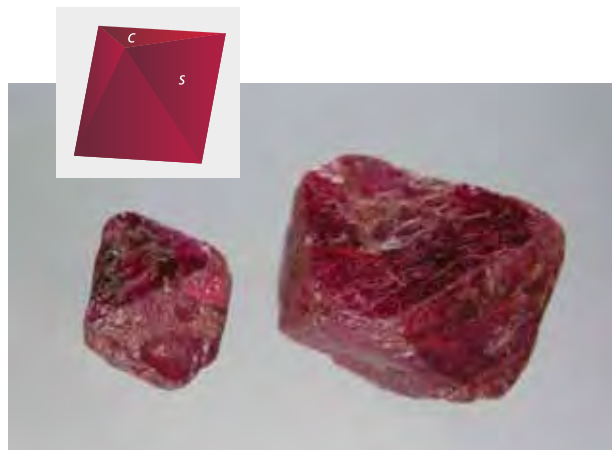
Figure 10. Most of the rhombohedral Winza ruby crystals (here, up to 13 \times 18 mm) showed negative rhombohedral (pseudo-octahedral) forms, consisting of s and c faces. Photo by K. Schmetzer.
