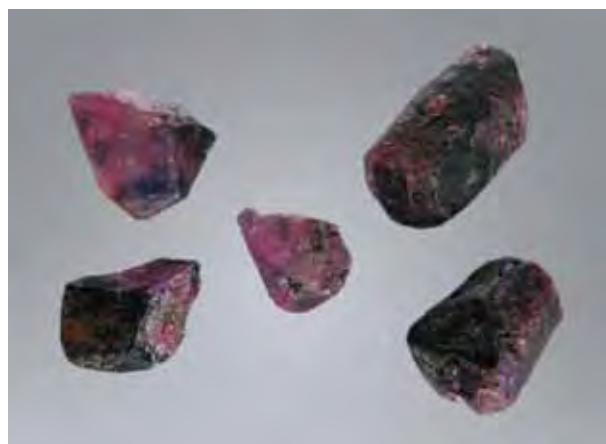
Figure 22. These corundum crystals have dark bluish violet- to black-appearing translucent to opaque phases exposed at their surfaces. The dark areas in the two crystals on the left were found to be blue-violet sapphire, the sample in the center (9 \times 12 mm) contained black amphibole, and the two samples on the right had a rim of black spinel. Photo by K. Schmetzer.
