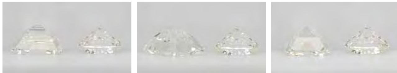
Figure 14. When grading fancy shapes, the average appearance is best represented by placing the fancy shape with its long axis approximately 45° to the observer. This series of photos for a 1.20 ct emerald cut next to a GIA master stone illustrate why this “middle” position is used. On the far left, the emerald cut is positioned so the observer views the long side—its weakest color appearance. The photo on the far right illustrates the appearance seen when the grader looks through the end of the fancy cut, where the color appears strongest. The angled position used at the laboratory, which averages the color, is seen in the center. Other fancy shapes also best simulate the outline of the round when set in this position. Photos by Robert Weldon.
