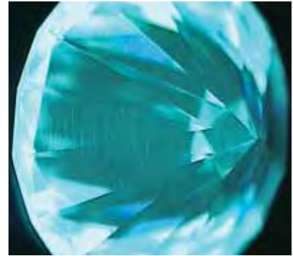
Figure 7. DiamondView imaging of the synthetic diamond shows blue-green fluorescence with yellow-green striations, consistent with reports for HPHT-treated CVD synthetic diamonds.
