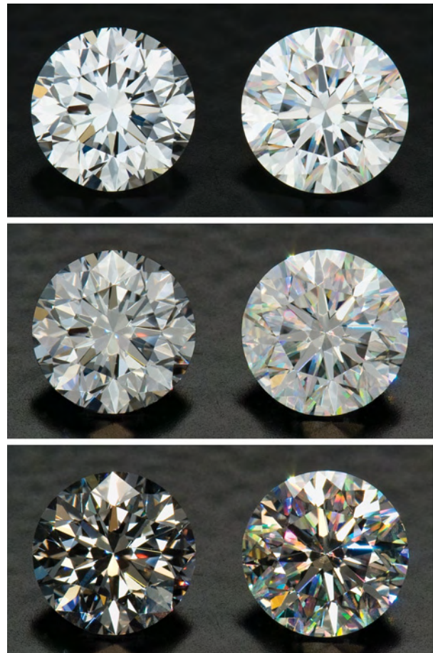
Figure 14. These two diamonds of similar proportions, one cut conventionally (RD01, left) and the other with pattern C (no. 32, right), are shown in three lighting environments: diffused (top), mixed (center), and spot lighting (bottom). When spot lighting is substantial, careful placement of the diffraction grating can improve the appearance of certain diamonds by making them more fiery. Photos by Robert Weldon.
