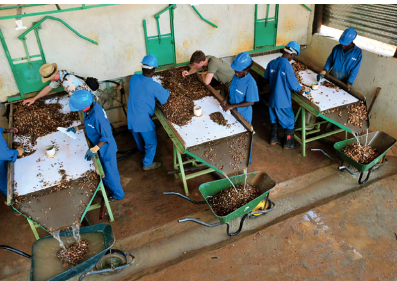
Figure 18. At the Mozambique Gems processing plant, the washed gravels are placed on white tables for hand picking of the tourmaline. Photo by V. Pardieu.
