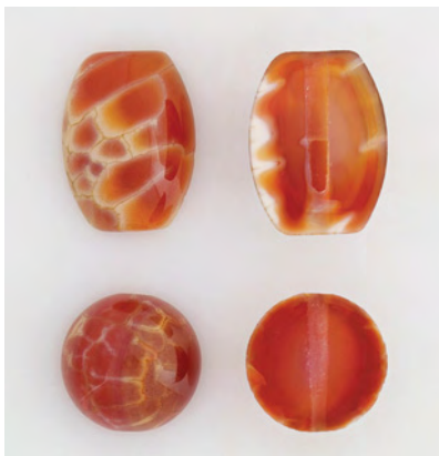
Figure 3. These two chalcedony beads were cut in half. Note that the fractures in the oval bead, where the white lines are more distinct, are significantly deeper and the white zones terminate with the fractures. The round bead is ~12.0 mm in diameter.
