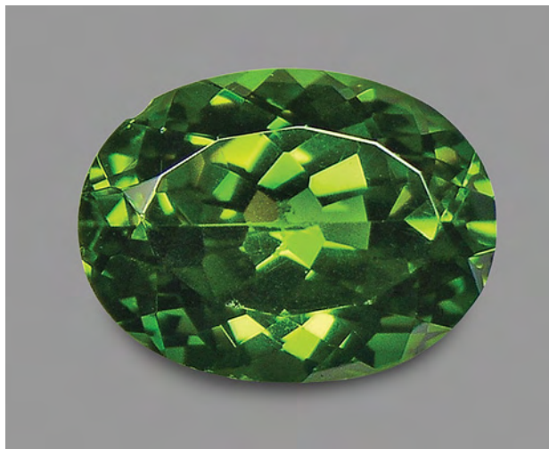
Figure 25. This brilliant, dispersive green sample, sold as peridot, is actually a barium-rich glass. Photo by T. Hainschwang.
