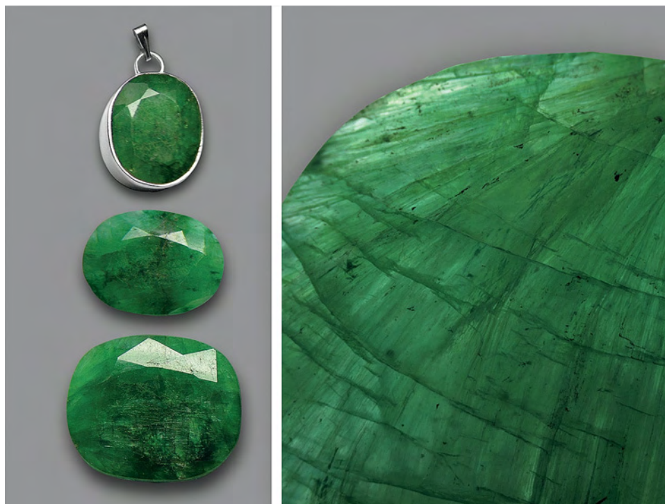
Figure 29. These three dyed sillimanites were represented as emeralds (left). With magnification, their fibrous structure showed green color concentrations, indicating the presence of dye (right, image width 11.5 mm). Photos by T. Hainschwang.
