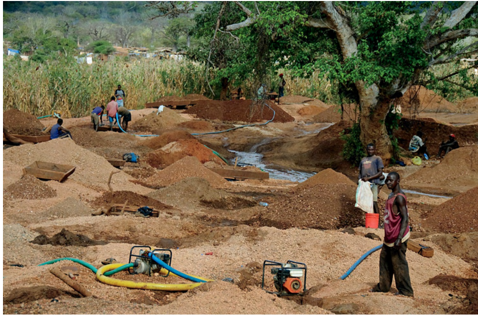
Figure 18. Rubies and sapphires from the Winza deposit in central Tanzania are recovered from primary deposits as well as from eluvium, which is wet-sieved using water from the adjacent seasonal river. The miners employ portable gasoline-powered pumps to make pools of water during times of low rainfall, as in this June 2008 photo. Photo by Brendan M. Laurs.
