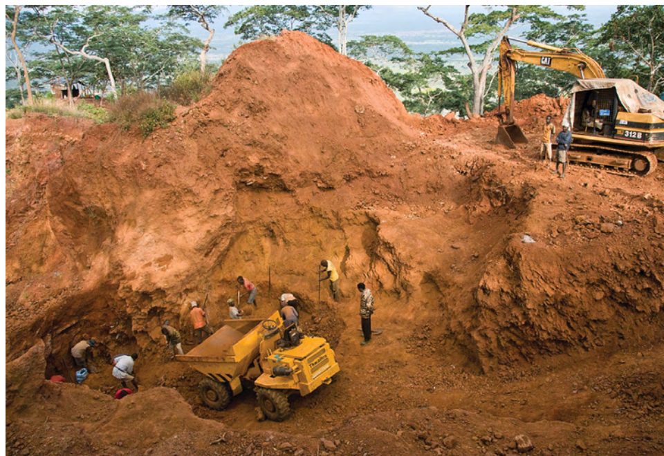
Figure 4. Open-pit mining for chrysoprase and prase opal is performed using an excavator and hauling vehicle. Photo by B. M. Laurs.
