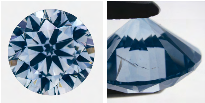
Figure 10. This 1.53 ct Fancy Intense blue round brilliant was found to be a type IIb HPHT-grown synthetic diamond. Patchy color zones and a fracture can be observed in the pavilion (right).
