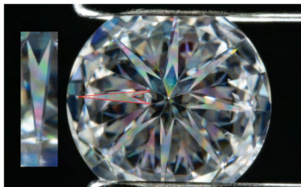
Figure 11. The grating patterns on the pavilion of this diamond (at 10 \times ) cover too much of the areas that normally reflect white light. This experimental pattern (A in figure 4) improved fire, but the overall appearance of the diamond was not as bright, and the contrast pattern was greatly diminished. Note that even though the diffraction grating creates spectral colors (inset at 30 \times ), the individual lines of the grating pattern cannot be seen, and areas that have been etched could be mistaken for unpolished or poorly polished facets. Composite photo by Robison McMurtry.
