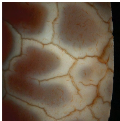
Figure 2. Magnification revealed that the white lines followed fractures in a pattern typical of quench crackling. Field of view ~5.3 mm high.
