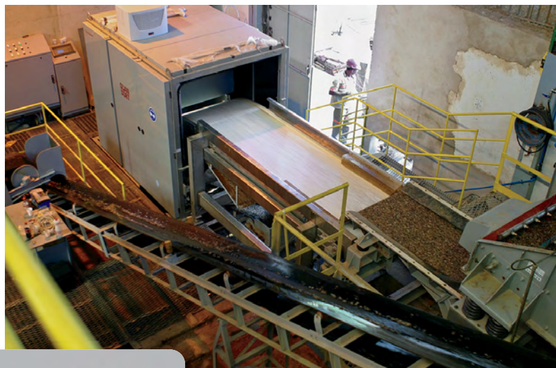
Figure 9. Near Nova Era in Minas Gerais, Brazil, the Belmont mine operates using sophisticated optical sorters and other machinery to ensure an efficient and steady
