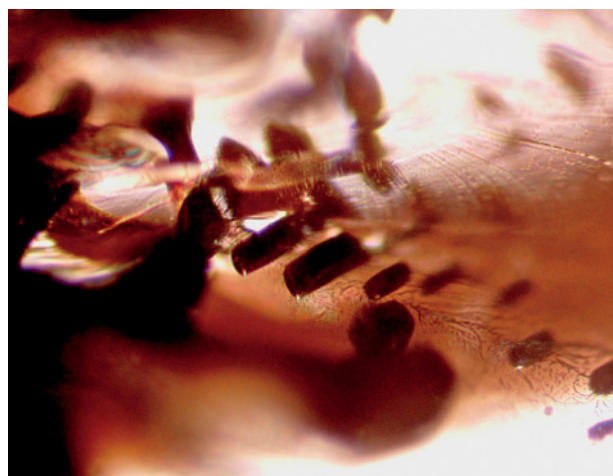
Figure 6. This group of magnetite inclusions in zircon occurred as short, parallel prisms. Photomicrograph by T. Chen; magnified 200×.
