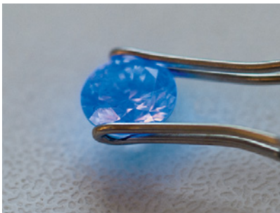
Figure 4. This colorless type IaB diamond (~0.75 ct) was cooled in a liquid-nitrogen bath during 325 nm laser PL analysis. When the stone was removed and warmed to room temperature, it briefly displayed a blue thermoluminescence emission.
