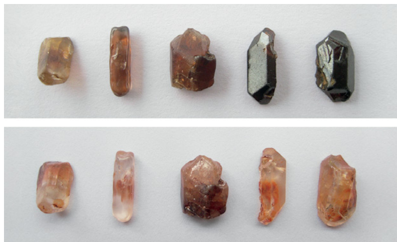
Figure 9. These Muling zircon samples (0.49–0.77 g), shown before and after heating, became significantly lighter after heat treatment. Photos by Y. Liu.
