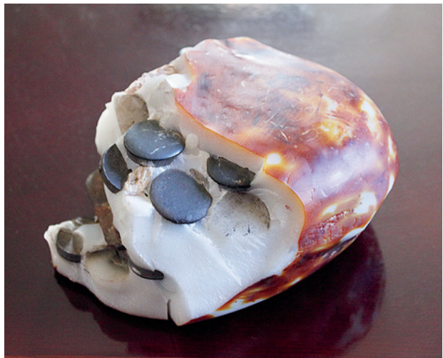
Figure 33. When broken open, this imitation nephrite sample (originally 12 x 9 x 6 cm and weighing 3 kg) was found to contain steel disks embedded within the surrounding material. Photo by Y. Zhang.
