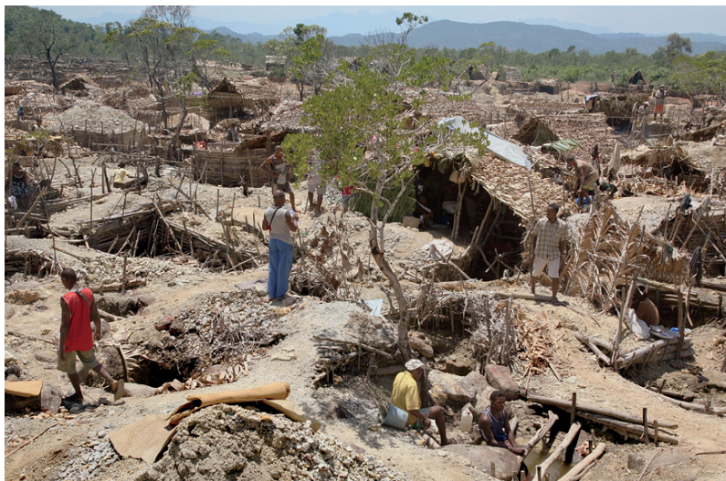
Figure 5. Thousands of miners have dug numerous pits in search of demantoid at the Antetetzambato deposit. Because of the tidal influx, they must carefully reinforce their diggings and pump seawater out of the pits before mining can resume each day. Photo by F. Pezzotta, November 2009.
