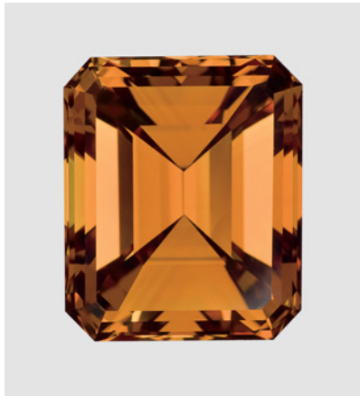
Figure 1. This 28.65 ct Fancy Deep brownish yellowish orange diamond is HPHT treated. The starting material was probably a typical cape diamond with light yellow or brownish yellow color.
