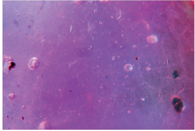
Figure 42. Trapped bubbles of various sizes demonstrate the extent of lead-glass filling in the trapiche ruby. Dark-colored inclusions, presumably apatite, are visible on the right. Photomicrograph by O. Segura; magnified 20×.
