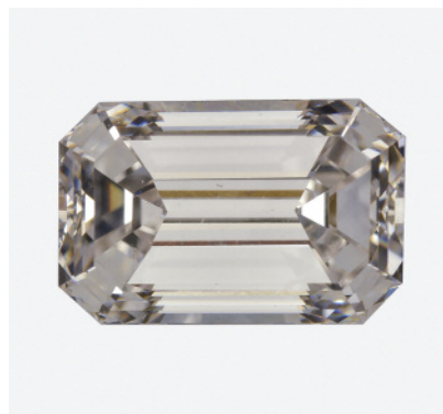
Figure 14. This 1.03 ct CVD synthetic is notable for its size and faint pinkish brown color.
