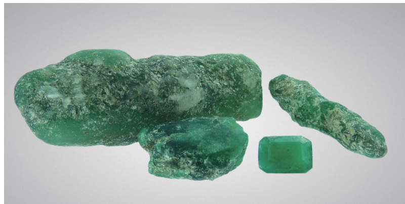
Figure 18. This massive Cr-muscovite, reportedly from southern Ethiopia, is better known in the trade as fuchsite. The longest rough piece measures 53 mm, and the faceted stone weighs 2.56 ct. The material was difficult to polish because of its low hardness, 3 or less on the Mohs scale. Photo by Thierry Pradat.
