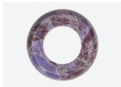
Figure 9. This 13.60 mm mottled purple bead consists primarily of jadeite and quartz.
