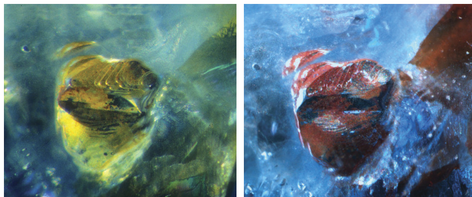
Figure 2. Left: This Sri Lankan sapphire hosts a blocky iron sulfide inclusion with a surface-reaching crack, both of which are coated with yellow limonite. Right: After heating in air to 350°C, the limonite coating on both the sulfide and the related fracture changed to rust-colored hematite. Photomicrographs by J.I. Koivula; magnified 10x.
