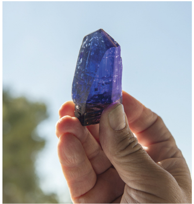
Figure 16. Tiny calcite crystals adhering to the surfaces of this superb tanzanite crystal, along with the brown coloration around its base, are strong indicators that the material has not been heated. The crystal weighs 500.45 ct and measures approximately 8 cm in length. Photo by Eric Welch; courtesy of New Era Gems.
