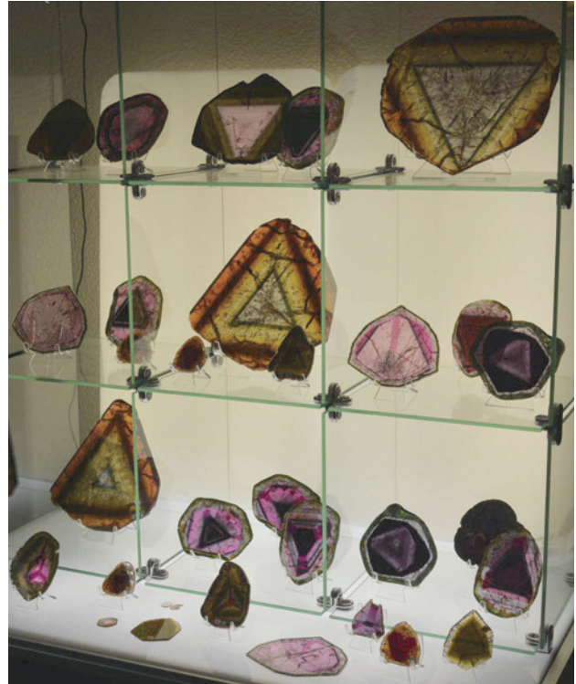
Figure 39. These slices of liddicoatite tourmaline display colorful growth zoning. The largest slice measures approximately 30 cm. Photo by Duncan Pay; courtesy of Frederic Gautier, Little Big Stone.
