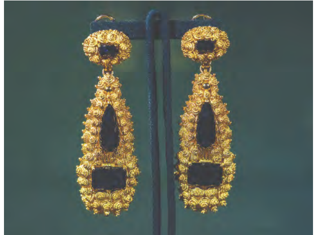
Figure 9. This pair of earrings is from an award-winning filigree inlay jewelry suite by Master Bai. Thin gold threads were bent to form springs, which were rolled to form the individual cones. Craftsmen then joined the cones to shape each earring before mounting the faceted jadeite. This filigree technique, known as piling, gives the pieces a light, airy feel. Photo by Eric Welch, courtesy of Zhaoyi Xintiandi (Beijing) Jewelry Co., Ltd.
