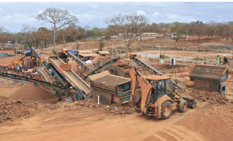
Figure 15. After the gravel passes through a grating, conveyor belts carry it through the washing stages until the ruby is finally trapped by the sluices. Photo by Vincent Pardieu/GIA.
