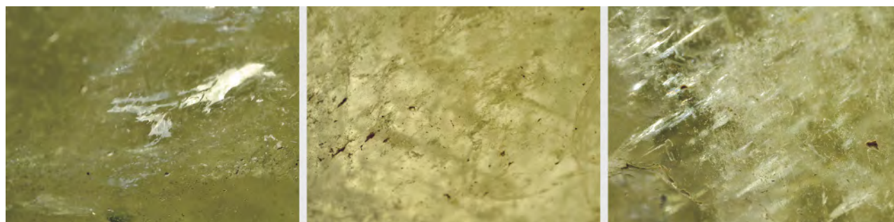
Figure 69. Examination of the carving with a hand loupe revealed reflective liquid films (left), elongated phase/short tubes oriented in one direction and aligned in planes intersecting each other at approximately 65/115^\circ (center), and parallel reflective films that appeared to be incipient cleavage (right). Photos by Gagan Choudhary; image width 25 mm.
