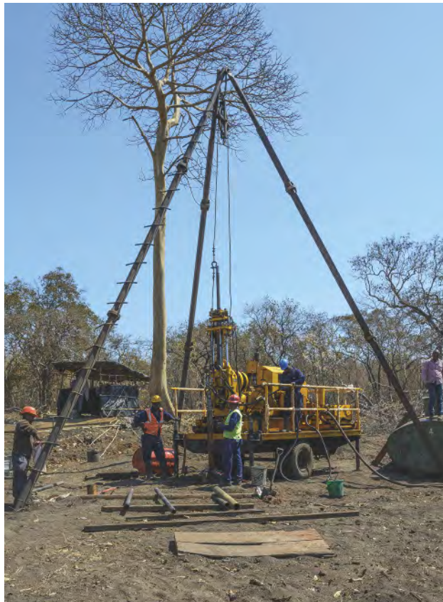
Figure 13. The setup of the core-drilling instrument. Water from a tank next to the working platform is run the whole time to cool the drill bit. Photo by Andrew Lucas/GIA.
