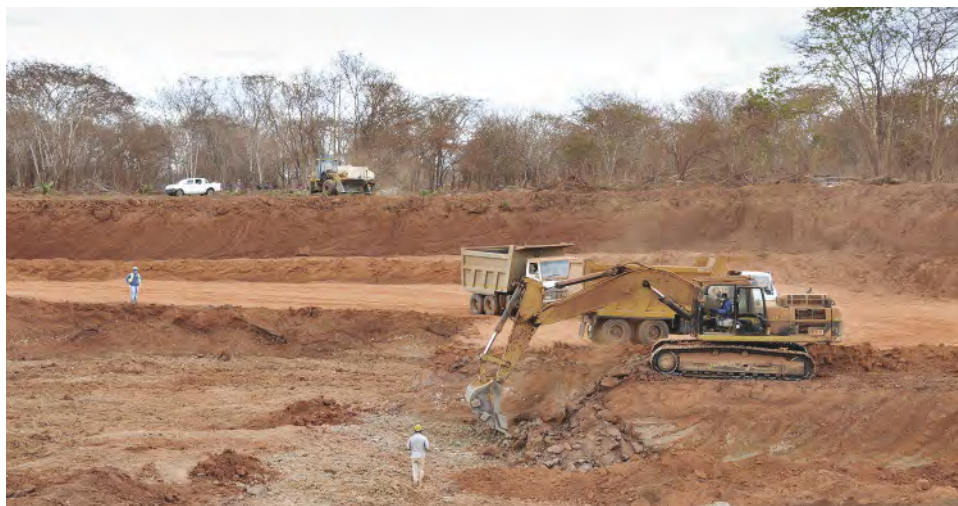
Figure 9. In the secondary deposit at pit 3, excavators and trucks work together to strip the overburden, load the ruby-bearing gravel, and transport it to the washing plant. Photo by Vincent Pardieu/GIA.
