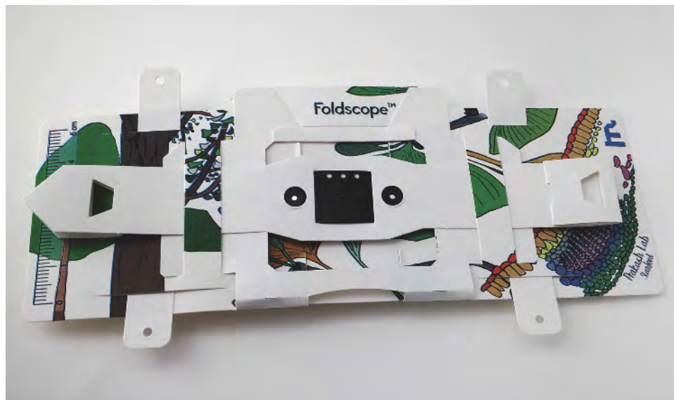
Figure 93. A fully assembled Foldscope measures approximately 7 × 2.5 in. A toggled LED light source is tucked into tabs on the back, and the bottom center slit accommodates standard glass microscope slides. Photo by Kate Pleatman.
