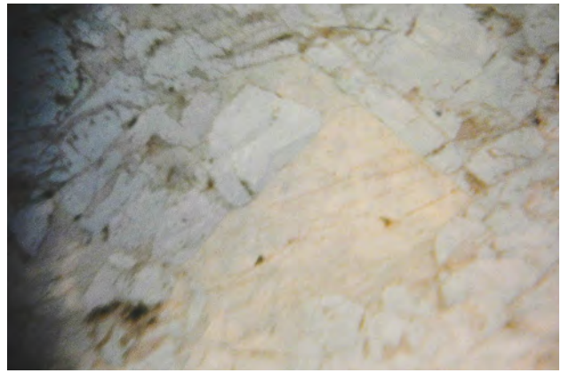
Figure 78. Two groups of minerals were observed on the surface of this sample under brightfield illumination. One group is composed of the pale whitish subhedral to euhedral grains, the other of the creamy minerals in between. Photomicrograph by Li Jianjun; magnified 30x.
