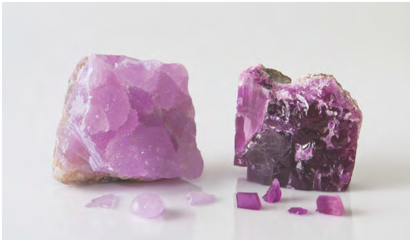
Figure 1. The pink and reddish purple cobaltocalcite specimens (246.3 and 361.0 g, respectively) are shown with some of the wafers cut from them.
