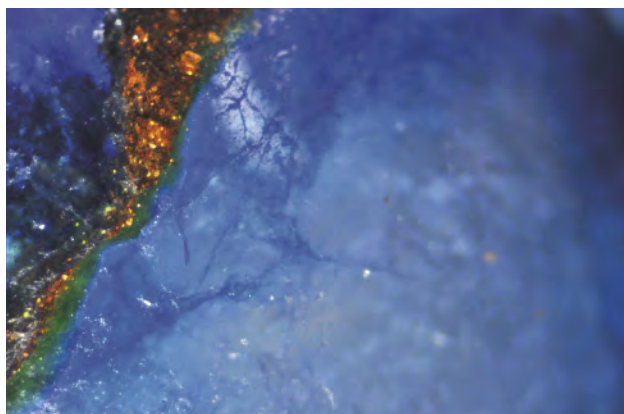
Figure 89. Color concentrations of blue dye were easily visible along the fractures against a white background, while the golden brown areas were composed of copper-zinc based fine flakes. Also note the greenish polymer along the edge of the golden brown and blue areas. Photomicrograph by Gagan Choudhary; magnified 48x.
