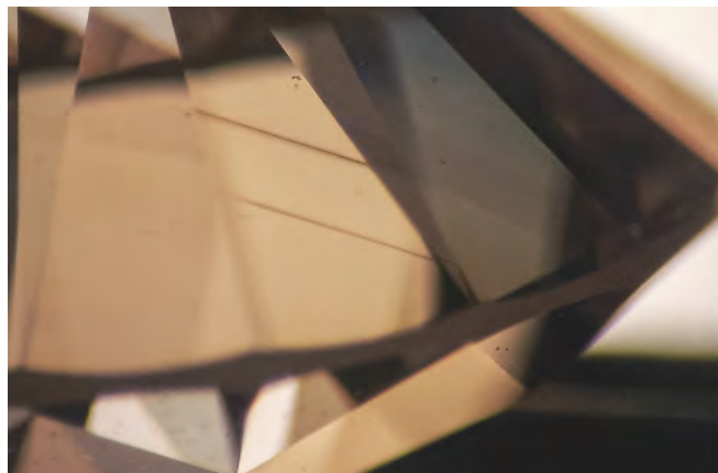
Figure 90. Left: These growth planes were observed in a CVD synthetic diamond; fine pinpoints were found along the growth planes. Photomicrograph by Meenakshi Chauhan; magnified 30x. Right: Pinpoints along the growth plane were also visible from the table. Photomicrograph by Meenakshi Chauhan; magnified 10x.
