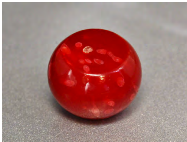
Figure 18. This 37.50 ct plastic bead contained visible fragments of carbonate-type coral (the lighter spots). Photo by Gagan Choudhary.
