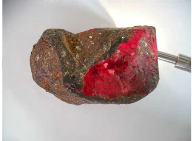
Figure 16. The rock crystal shows dark red under transmitted light to imitate ruby. Photo by Nazar Ahmed Ambalathveettil, Dubai Central Laboratory.
