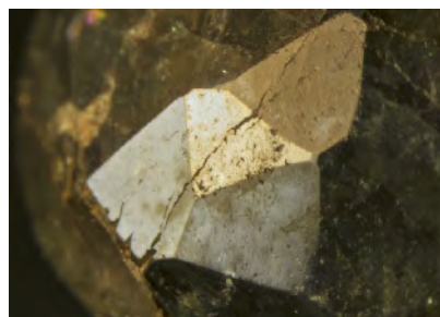
Figure 16. Diffused reflected light exposed spotty luster on the surface of one of the tested stones, indicating the presence of a coating. Field of view 2.17 mm.
