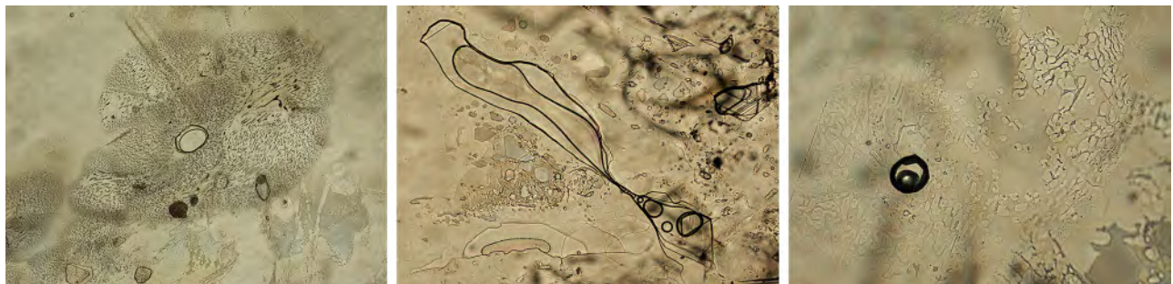
Figure 14. Left: A two-phase glassy melt and gas inclusion and a glass-filled discoid fracture in a sapphire from the Rock Creek deposit in Montana. Center: A two-phase glassy melt and gas inclusion and a glass-filled discoid fracture in a sapphire from the Rock Creek deposit. Right: A two-phase glassy melt and gas inclusion, in a sapphire also from the Missouri River, showing the surrounding discoid fracture. This fracture presumably filled with a silicate liquid and partially healed, leaving an impression in some places of the corundum host’s trigonal crystallographic orientation. Photomicrographs by Aaron Palke; field of view 1.24 mm (left) and 0.62 mm (center and right).
