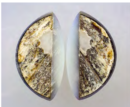
Figure 19. Left: The cross-section revealed the white fluted object with a spiderweb structure bordering the shell base. Right: DiamondView imaging showed a moderate white blue reaction following the spiderweb pattern.
