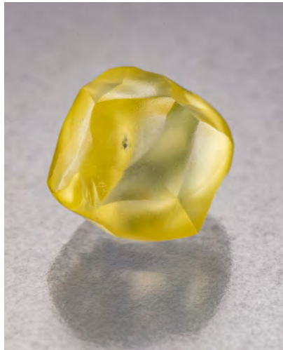
Figure 2. This 2.47 ct rough diamond was HPHT processed to improve its color. Unlike conventional HPHT-treated diamonds, this stone has a natural-looking surface.
