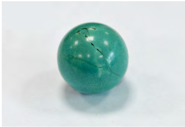
Figure 25. Spectroscopic analysis of this 15.21 gram turquoise reveals that the material has been both impregnated and dyed. Photo by Wen Han.
